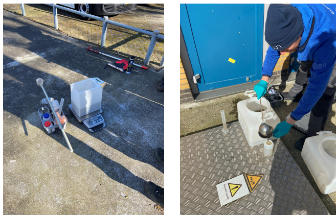
Figure 9.4: The equipment needed for taking samples (right) and the filling of a jar with collected wastewater (left).
