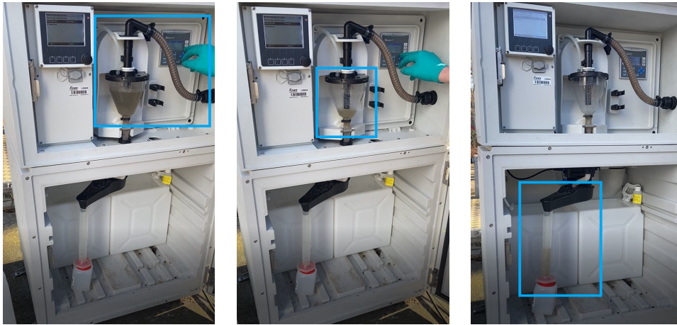
Figure 9.2: The process of sampling: filling of the flask (left), measurement of an aliquot (middle), flow of the aliquot through the carousel (right). The pictures are taken during the sampler's work to determine the aliquots volume.
