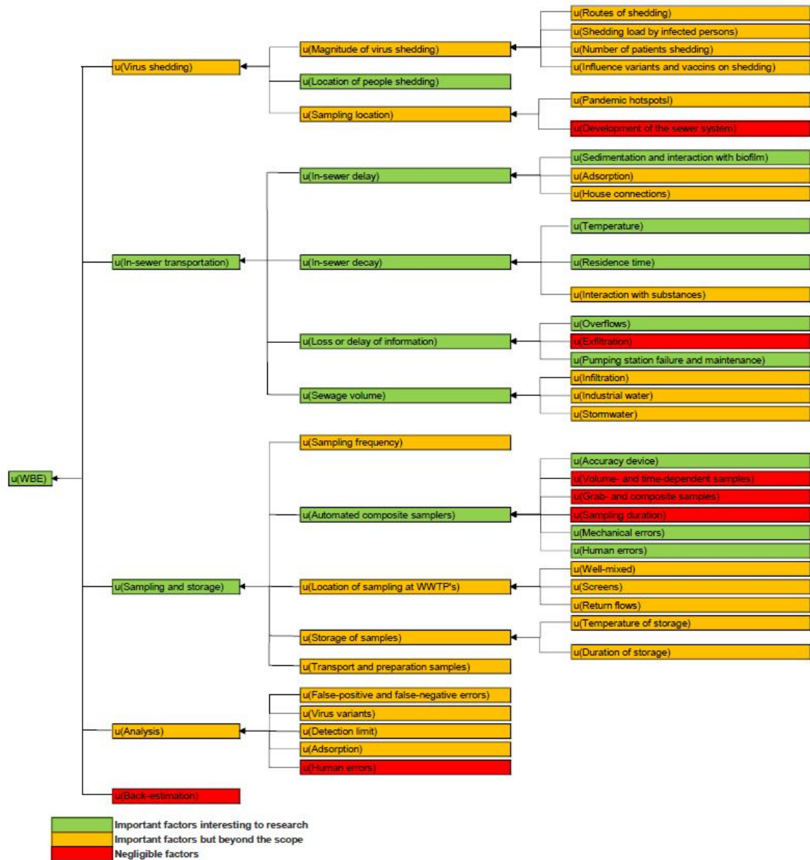
Figure 2.3: Conclusion on the literature review. This dendrogram presents the factors that are investigated quantitatively in this thesis. Green is showing relevant factors that are interesting for this research, orange are interesting factors but beyond the scope of this thesis and red is showing negligible factors.
