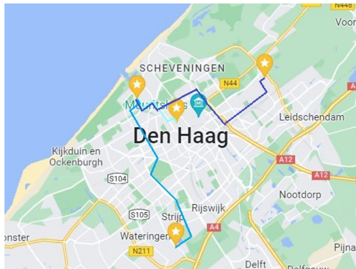
Figure 6.2: The locations in The Hague for which the residence time has been determined. The stars show the three locations, as well as WWTP Houtrust. The blue lines represent the flow direction to WWTP Houtrust.
