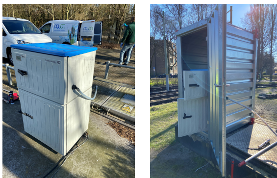
Figure 9.1: Automated composite samplers located in Delft (left) and at Leyweg, The Hague (right).
