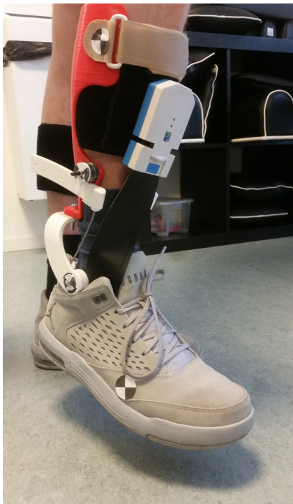
Figure 60: Patient prototype. the blue/grey block on the patient's shin is the transmitter of the pressure measuring insoles and does not belong to the prototype.
