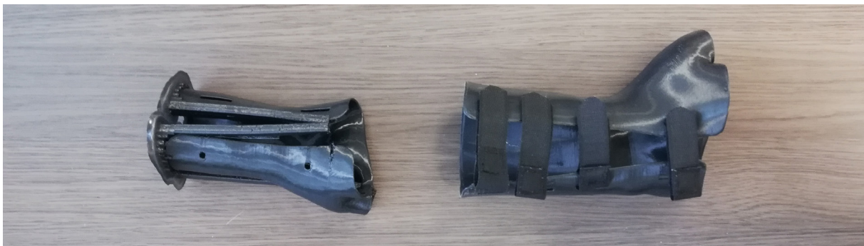
Figure 21: The raw wrist orthosis straight out of the printer (left) and a finished wrist orthosis (right).
