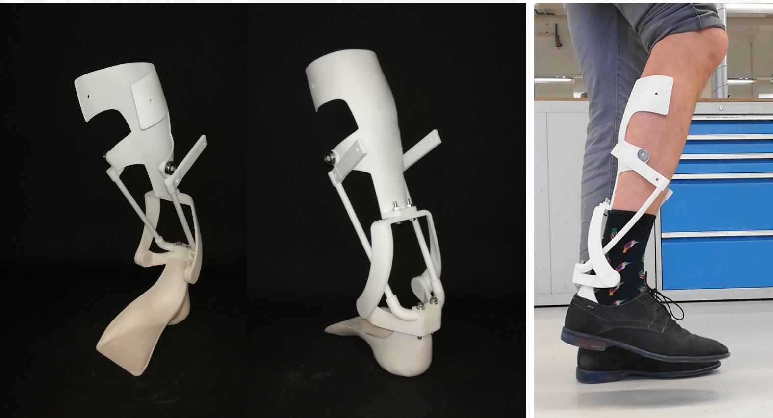
Figure 45: (left) The 3D first functional prototype. (middle) The neutral position during swing. (right) Performance measurement setup
