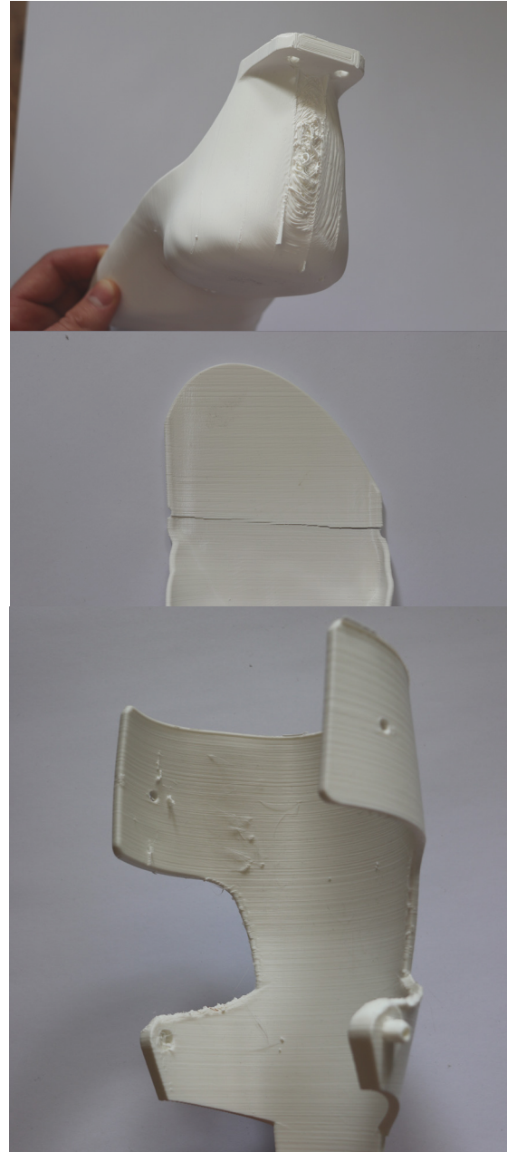
Figure 56: (top) FDM result after support removal, (middle) delamination of the toe plate and (bottom) imperfect surface finish (bottom).
