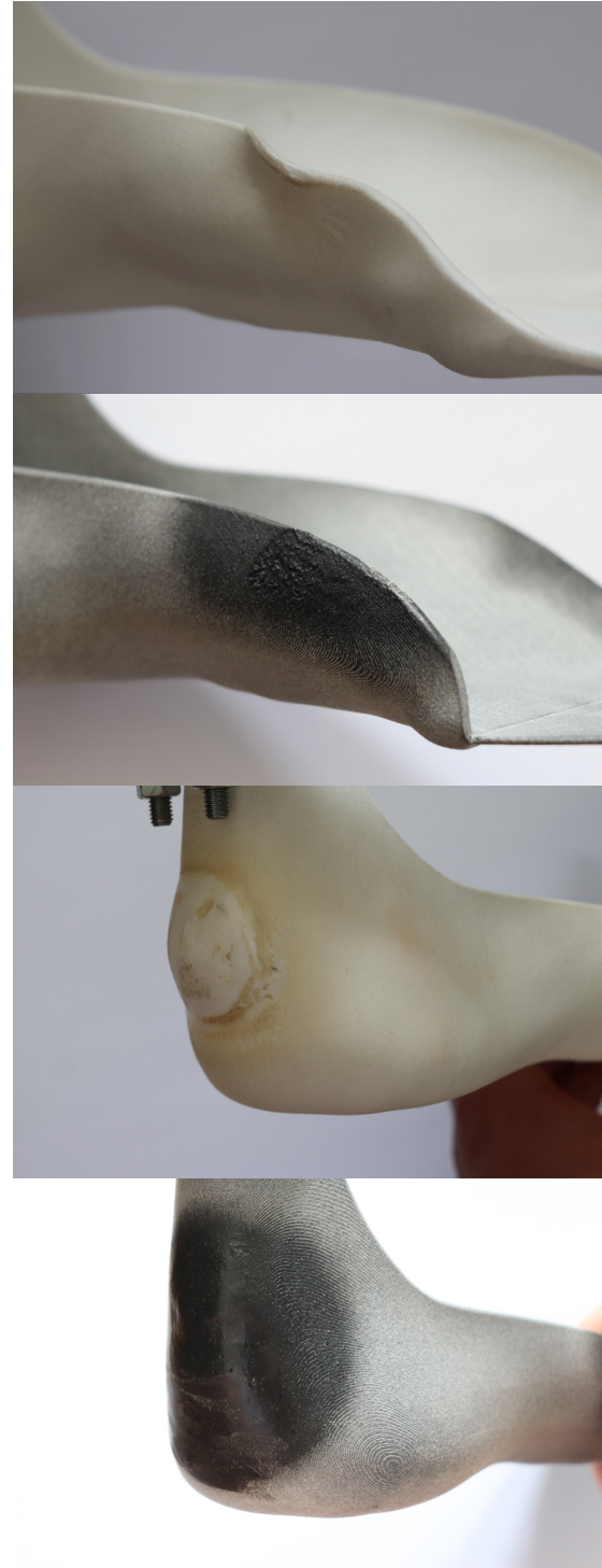
Figure 58: Deformed and sanded trim lines for SLS (top) and MJF (2nd from top). Deformed and sanded heel for SLS (3rd from top) and MJF (bottom).
