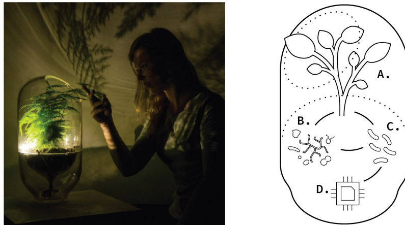
Figure 7. Image of Living Light lamp (Van Oers & Plant-E, 2016) (left) and a visual interpretation of multispecies interactions within (right); A. Plant (asparagus); B. Soil microbes (various species); C. Electron-producing bacteria ( Geobacter sulfurreducens ); D. Digital system (cathode, anode, sensor, processor, LED).
