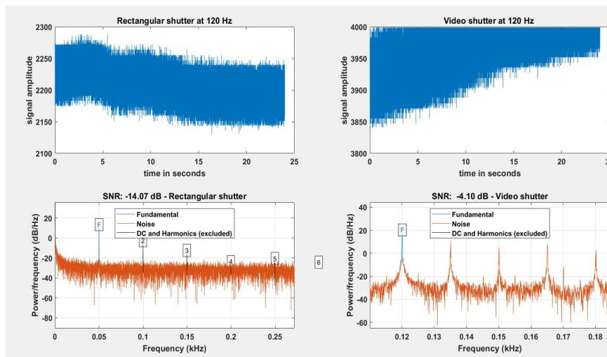
Figure 6.13: Received signal and power spectral density of the shutters.
