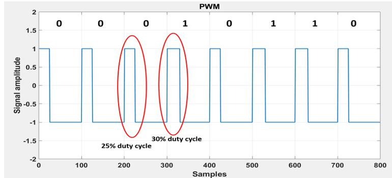
Figure 5.8: Pulse Width Modulation (PWM).
