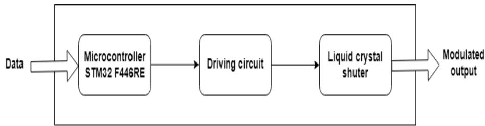
(a) Block diagram of the transmitter
