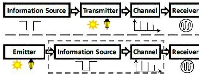
Figure 2.2: Communication channel standard (above) and passive (below) [23] .
