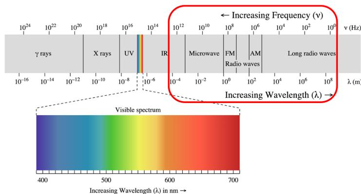
Figure 2.1: Electromagnetic spectrum composition [12].
