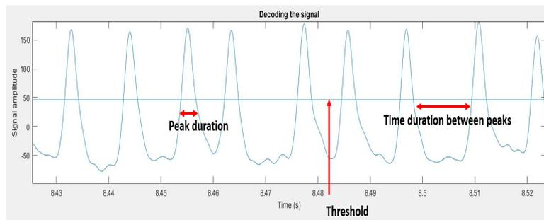
Figure 6.1: Signal measurements for decoding.
