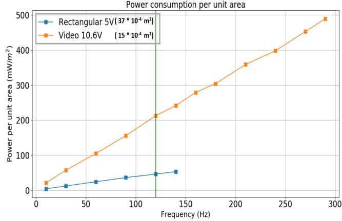
Figure 6.11: Power consumption per unit area.
