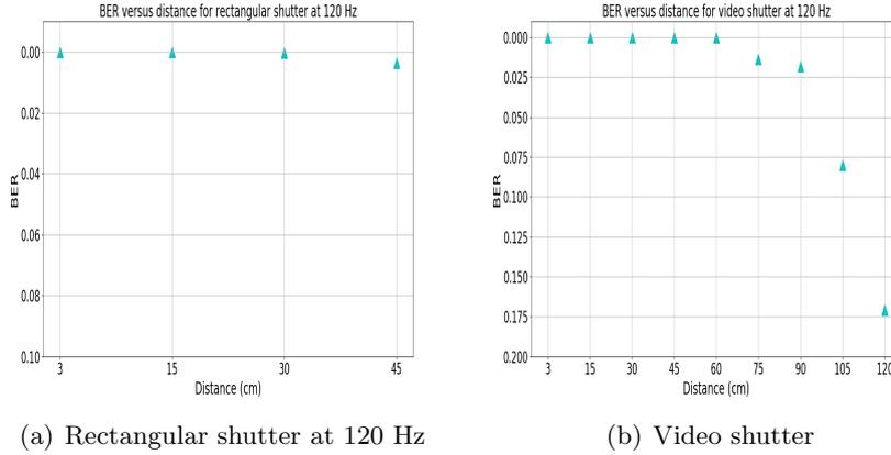
Figure 6.8: Distance v/s BER at 120 Hz.
