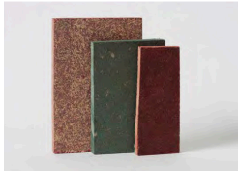
Fibreboard made from 100% wet meadow fibres Manufactured by Zelfo Technology GmbH
