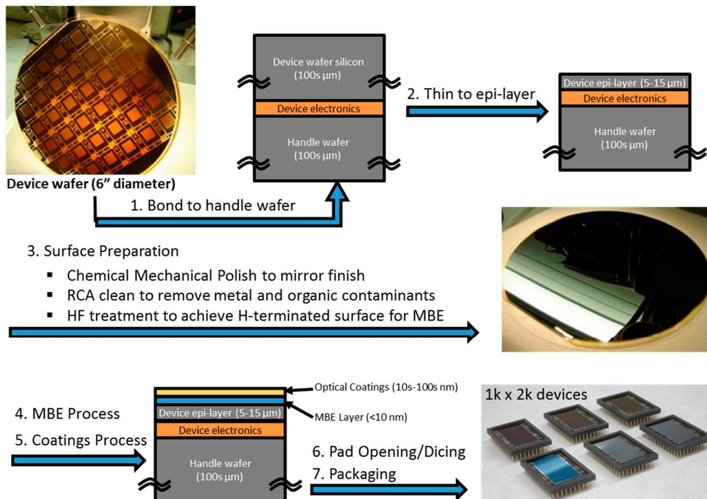
**Figure 4.** Process flow for end-to-end post fabrication processing along with schematic diagram of a superlattice-doped or delta-doped arrays (summarized as MBE layers), and the photographs of bare and AR-coated BSI silicon detector arrays. The coated arrays can be discerned from the reflective hue seen in photograph.
