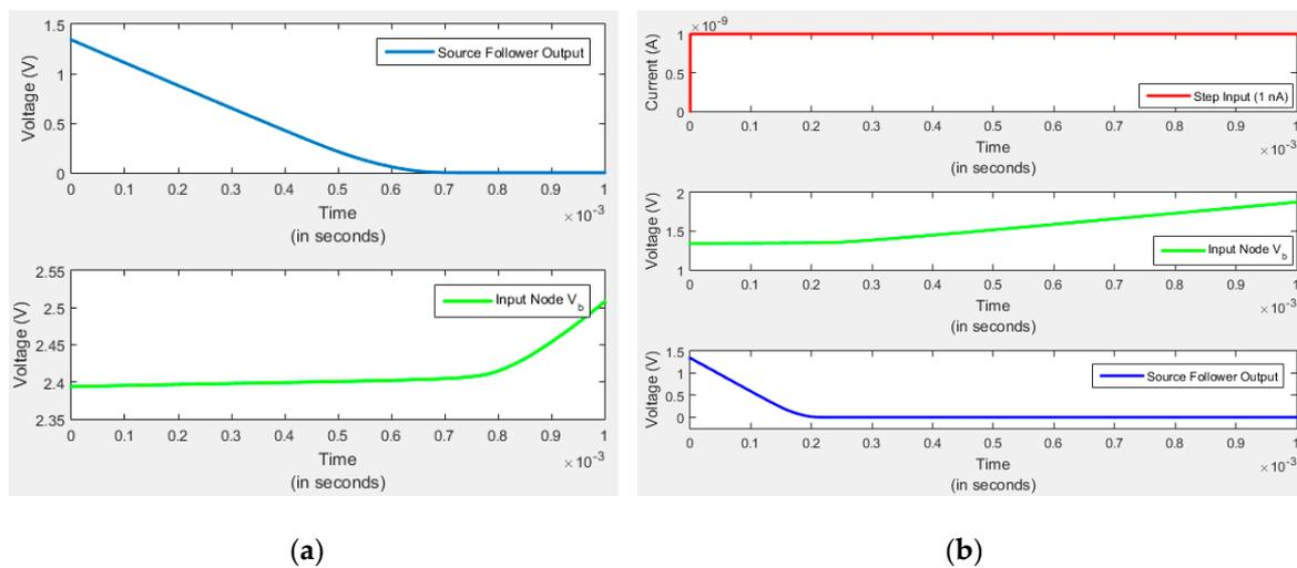
**Figure 17.** (a) As photodiode current starts to flow, the voltage at the node  $V_b$  rises from its initial value. As this occurs, the output voltage (source follower output) drops to 0. (b) A step response is simulated for a sudden increase in the input current from 0 to 1 nA. As soon as the input current rises to 1 nA, the output nodes settle to their steady state value without any ringing or overshoot.
