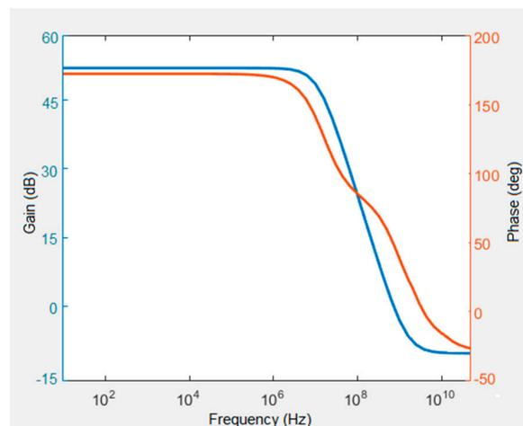
**Figure 18.** Frequency response of the readout circuit. The gain is around 45 dB with a 3 dB frequency of 10 MHz, close our target value. The modeling results indicate that the system operation is stable within the designed bandwidth.
