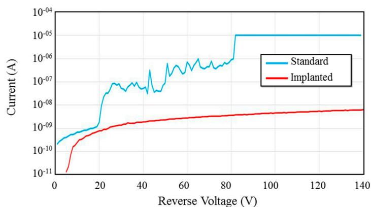
**Figure 14.** Current-voltage characteristics for an APD without contact-edge ion implantation (blue) and with implantation (red). Dark current and irreversible damage present in the unimplanted sample are reduced or eliminated by the implantation. First published in *IEEE Photonic Technology Letters* [51].
