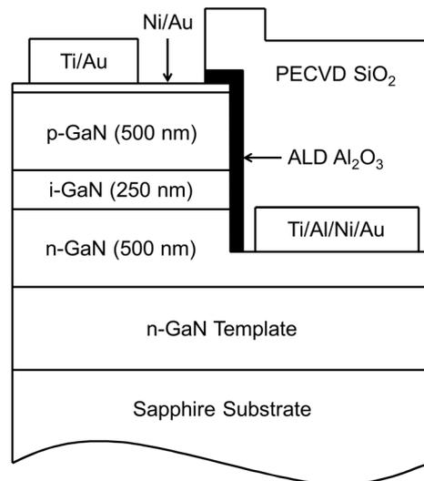
**Figure 7.** Schematic of device geometry showing the application of the ALD Al<sub>2</sub>O<sub>3</sub> layers as sidewall passivation and incorporating PECVD SiO<sub>2</sub> as a contact isolation layer. In devices not receiving the ALD treatment, the mesa sidewalls are passivated by the PECVD film only.
