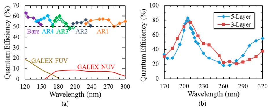
**Figure 9.** (a) QE data of delta-doped conventional (closed diamonds) and EMCCDs (open diamonds) enhanced with single layer AR coatings [34]. (b) QE data from two superlattice-doped CCD201s (e2v's 1k × 2k EMCCD) optimized for the 200–220 nm wavelength range; the device designs included a three-layer AR coating (red squares) and a five-layer AR coating (blue diamonds).
