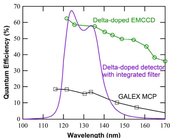
**Figure 3.** Model performance of a 2D-doped detector with an integrated visible-blind bandpass filter for far UV wavelengths. The multilayer MDF was designed to provide high in-band QE, and high out-of-band rejection ( $>10^4$ ). As designed the MDF includes layers of  $\text{MgF}_2$  (20 nm thick), Al (26 nm),  $\text{MgF}_2$  (18 nm), Al (20 nm), and  $\text{MgF}_2$  (11 nm), starting from the silicon interface up to the air interface.
