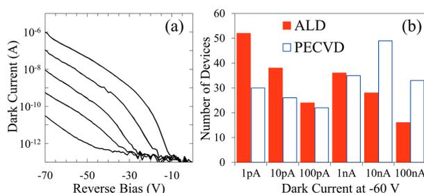
**Figure 12.** (a) Example of the variation in reverse bias behavior observed for ALD-passivated GaN APDs; (b) Histogram of  $\sim 200$  devices with 25- $\mu$ m diameter samples receiving a sidewall passivation layer of ALD Al<sub>2</sub>O<sub>3</sub> or PECVD SiO<sub>2</sub>. First appeared in *MRS Proceedings* [50].
