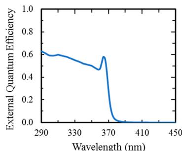
**Figure 11.** External QE as a function of photon wavelength for an Al<sub>2</sub>O<sub>3</sub>-passivated GaN p-i-n APD with zero applied voltage. With no applied voltage, there is unity internal gain.
