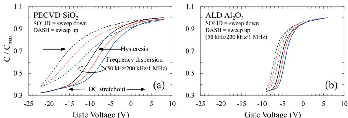
**Figure 13.** High-frequency CV characteristics for MOS capacitors fabricated on n-type GaN. A large reduction in the qualitative indicators of charge trapping—including voltage hysteresis, frequency dispersion, and stretchout—is observed for devices fabricated with (b) ALD  $\text{Al}_2\text{O}_3$  compared to those with (a) PECVD  $\text{SiO}_2$ .
