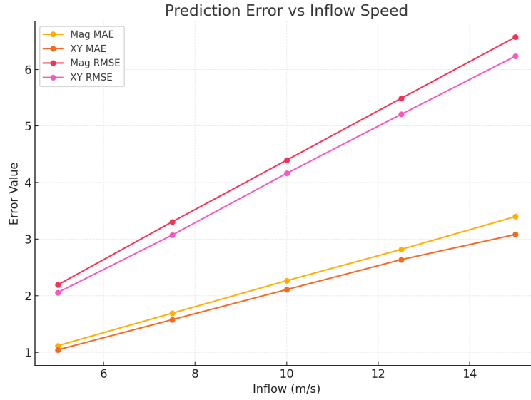
Figure 5.1: Prediction errors (MAE and RMSE) at different inflow speeds for models trained with magnitude and XY velocity inputs.
