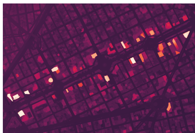
Figure 5. Individual buildings can be clearly seen in the 1.5-meter DSM from INEGI
