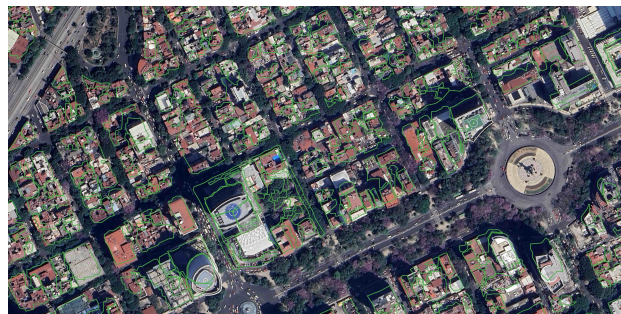
Figure 6. The building footprints that were created using the INEGI data. By taking advantage of the DSM data and not enforcing strict rectilinear polygons, the method creates reasonably accurate building footprints for complex buildings.
