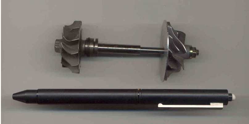
Figure 18.17 Micro turbine rotor with compressor and turbine
