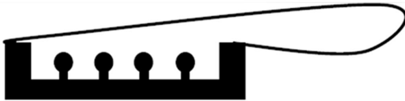
Figure 97: Water filled inflatable dam under the influence of flowing water.
