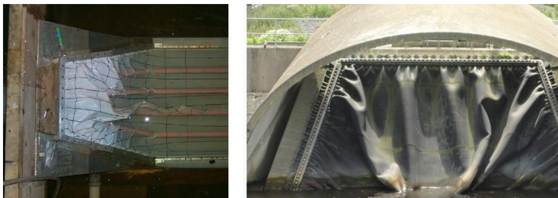
Figure 37: Fold formation above abutment in deflated state, Left: scale model, Right: Ramspol.
