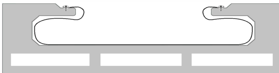
Figure 150: Bottom recess with holes in the bottom slab to reduce weight.
