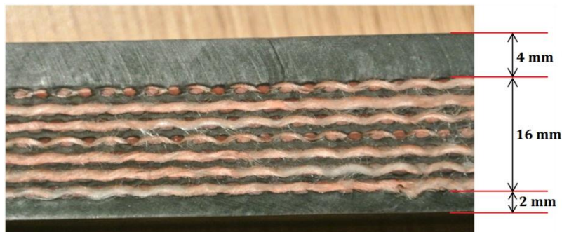
Figure 139: Dunlop Conveyor belting Superfort® 7 plies
