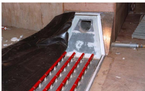
Figure 35: Scale model with rotating guide rollers (Photo WL | Delft Hydraulics).
