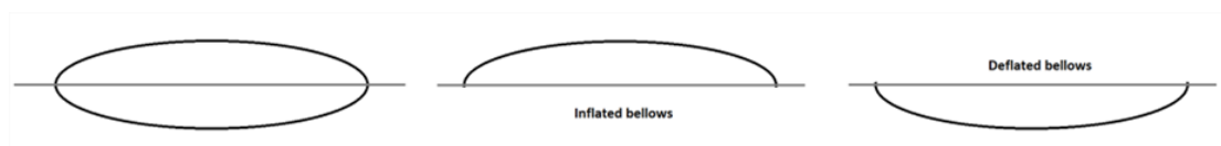
Figure 123: Longitudinal cross-section of an inflatable dam with a deep bottom recess.
