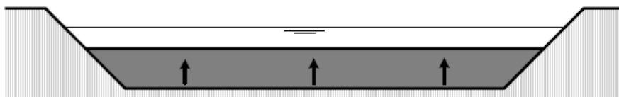
Figure 23: Cross-section of the water filled inflatable dam during inflation.
