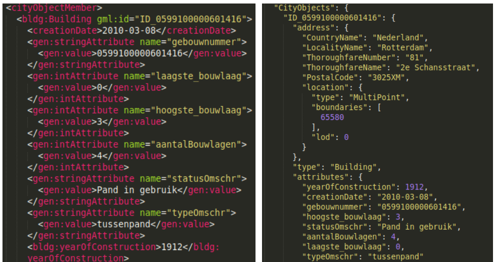
(a) A snapshot of a 3DCM file encoded in CityGML Source: Municipality of Rotterdam (originally in CityGML ) (b) A snapshot of a 3DCM file encoded in CityJSON Source: Municipality of Rotterdam (converted from CityGML )
