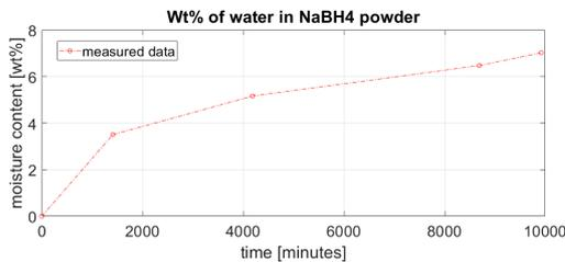
Fig. 11: Wt% of water absorbed by NaBH<sub>4</sub> powder in a closed container with an open water container inside.
