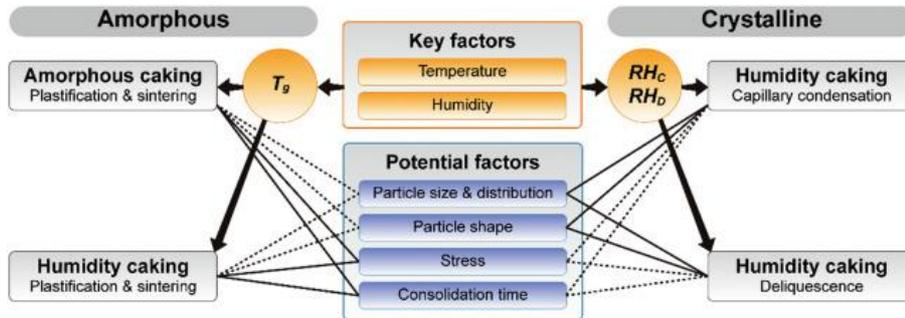
**Figure 4.** Factors of amorphous and humidity caking.  $RH_c$  is the required relative humidity to achieve capillary condensation, and  $RH_d$  that of deliquescence. Factors connected by a solid line are considered to be relatively more important than the ones connected by dotted line.
