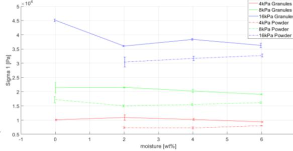
Fig. 7: Consolidation stress vs moisture content of  $\text{NaBH}_4$  granules and powder under varying normal stresses.
