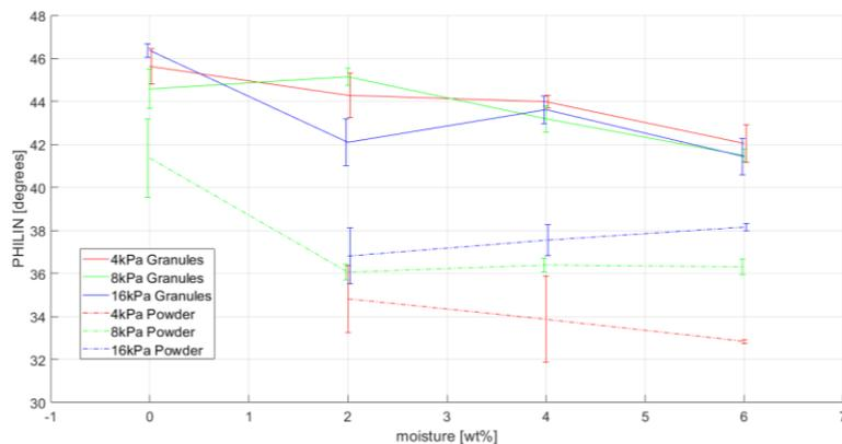
**Figure 25.** Slope angle of the linearized yield locus vs moisture content of NaBH<sub>4</sub> granules and powder under varying consolidation stresses.
