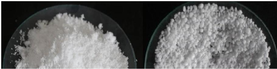
**Figure 5.** (left)  $\text{NaBH}_4$  powder, particle size 180-480 microns [24] and (right) granules, particle size 1.2 – 3.0 millimetres [25].
