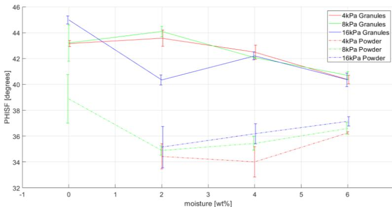
**Figure 26.** Angle of internal friction at steady-state flow vs moisture content of NaBH<sub>4</sub> granules and powder under varying consolidation stresses.
