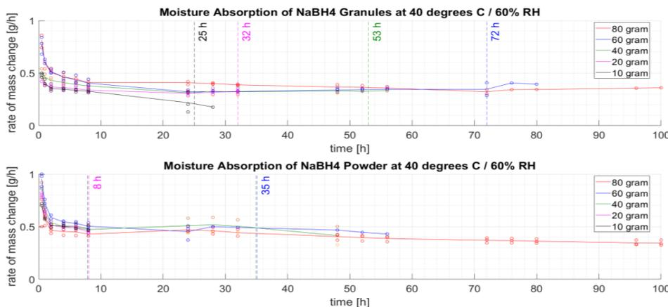
Fig. 6: The rate of mass change per hour of  $\text{NaBH}_4$  granules (top) and powder (bottom) when exposed to 40 degrees Celsius, 60% RH. The vertical lines indicate the average timestep at which moisture penetrated the bottom of the tube.
