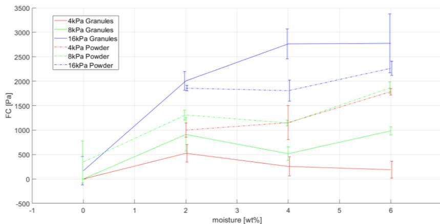
**Figure 23.** Unconfined yield strength vs moisture content of NaBH<sub>4</sub> granules and powder under varying consolidation stresses.
