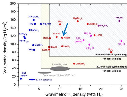
Fig. 1: Overview of various materials and their volumetric and gravimetric hydrogen density. The U.S. Department of Energy targets for hydrogen storage systems are also shown for comparison. [11]
