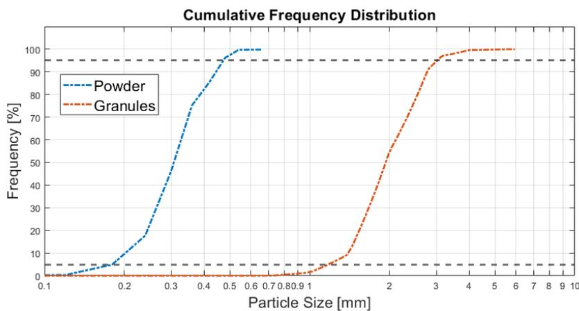
**Figure 6.** Average cumulative frequency distribution of  $\text{NaBH}_4$  granules and powder. The dashed horizontal grey lines represent the bracket which contains 90% of the cumulative frequency distribution. Data provided by M.C. van Benten.
