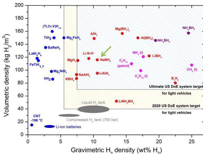
**Figure 1.** Overview of various materials and their volumetric and gravimetric hydrogen density. The U.S. Department of Energy targets for hydrogen storage systems are also shown for comparison. By K.T. Møller [8]
