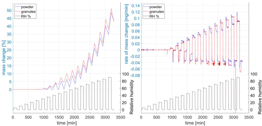
**Figure 14.** (left) Mass change over time and (right) rate of mass change, in % of original sample weight, of  $\text{NaBH}_4$  granules and powder when exposed to varying levels of ambient humidity. (The black lines in both show the relative
