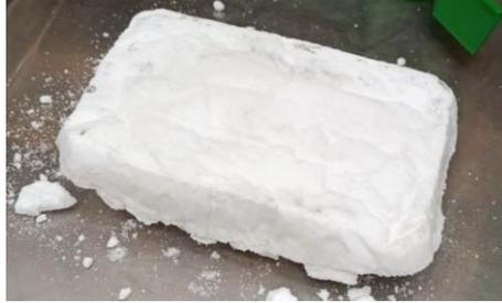
Fig. 12: Dried NaBH<sub>4</sub> powder after exposure to 5 wt% moisture.
