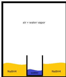
Fig. 4: Schematic overview of exposing  $\text{NaBH}_4$  to humidity in an enclosed environment.
