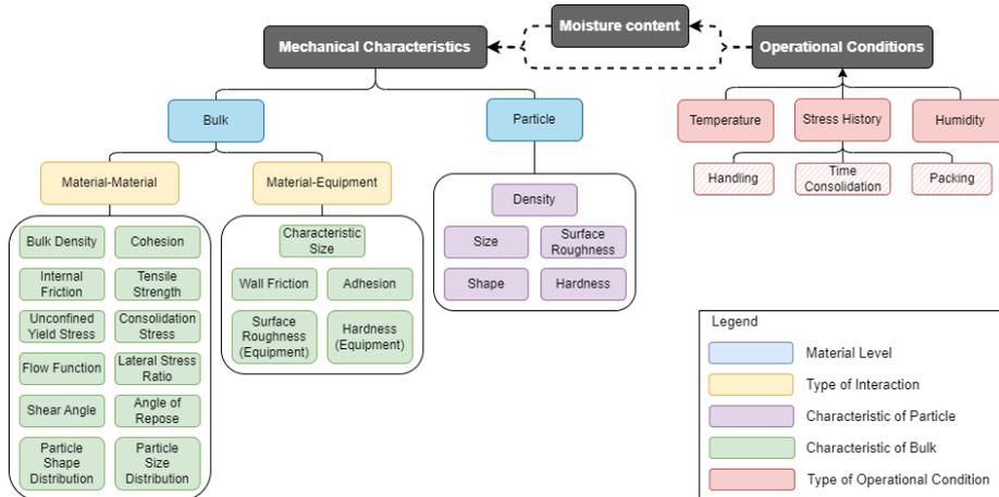
**Figure 2.** Most relevant mechanical properties of a material for storage and handling. Based on M.C. van Bente, [19]
