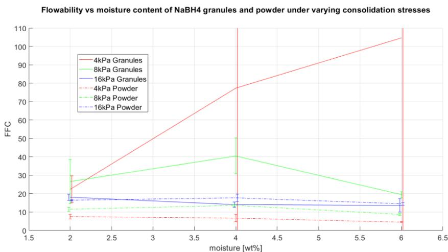
**Figure 24.** Flowability vs moisture content of NaBH<sub>4</sub> granules and powder under varying normal stresses. The confidence intervals of 4kPa Granules exceed the graph due to high uncertainty.
