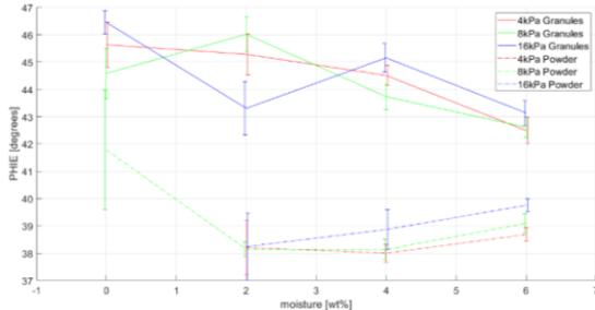
Fig. 10: Effective angle of internal friction vs moisture content of NaBH<sub>4</sub> granules and powder under varying consolidation stresses.
