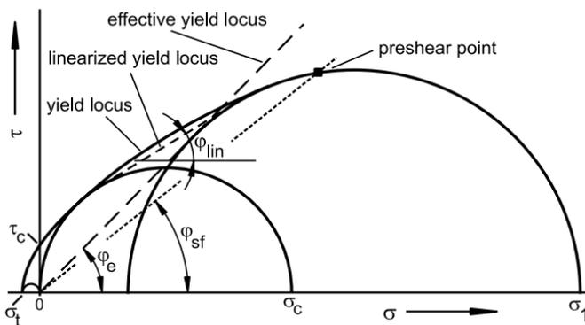
**Figure 20.** Mohr stress circle and its derived properties;  $\sigma_1$ , the consolidation stress;  $\sigma_c$ , the unconfined yield strength;  $\phi_{lin}$ , the slope angle of linearized yield locus;  $\phi_{sf}$ , the angle of internal friction at steady-state flow;  $\phi_e$ , the effective angle of internal friction;  $\tau_c$ , the cohesion; and  $\sigma_t$ , the tensile strength.
