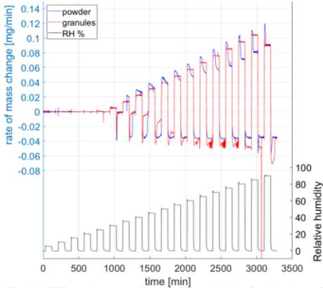
Fig. 5: DVS results: rate of mass change, in % of original sample weight, of  $\text{NaBH}_4$  granules and powder when exposed to varying levels of ambient humidity.
