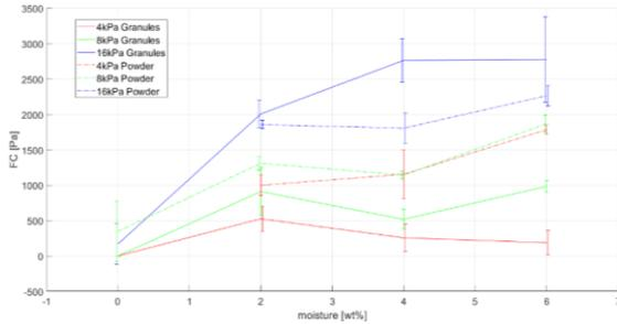
**Fig. 8:** Unconfined yield strength vs moisture content of NaBH4 granules and powder under varying consolidation stresses.
