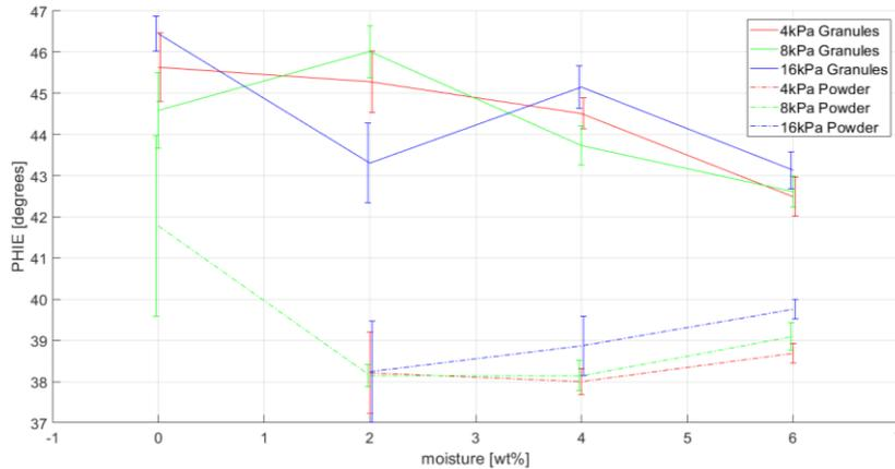
**Figure 27.** Effective angle of internal friction vs moisture content of NaBH<sub>4</sub> granules and powder under varying consolidation stresses.
