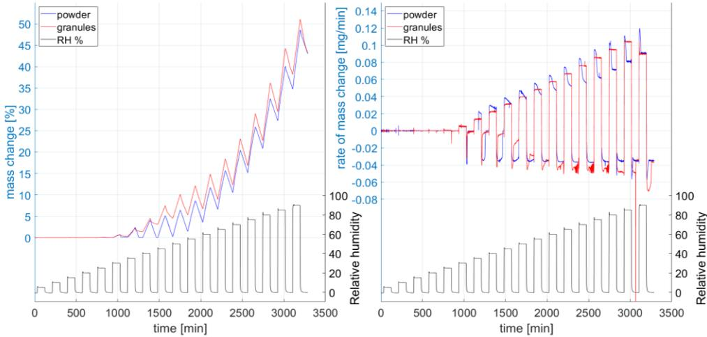
Figure 14 shows that the average rate of mass change for the powder at 25% RH is 1.5  $\mu\text{g}/\text{min}$ , while the granules have an average rate of mass change of 4.5  $\mu\text{g}/\text{min}$ . The rate of mass change becomes more noticeable at 30% RH and keeps increasing linearly from that point forward up to 0.1 mg/min at 90% RH.
