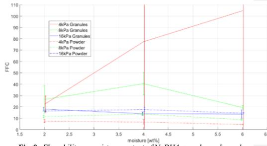
**Fig. 9:** Flowability vs moisture content of NaBH4 granules and powder under varying normal stresses. The confidence intervals of 4kPa Granules exceed the graph due to high uncertainty.
