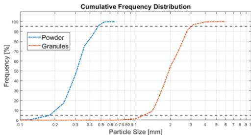
Fig. 3: Average CFD of  $\text{NaBH}_4$  granules and powder. The dashed horizontal grey lines represent the bracket which contains 90% of the CFD. Data provided by M.C. van Benteen.
