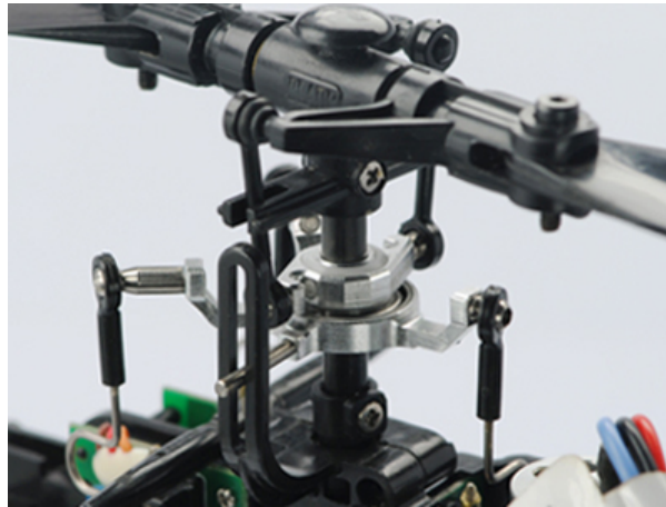
Figure 11.2: An Example of a Small-Scale Swashplate System a
