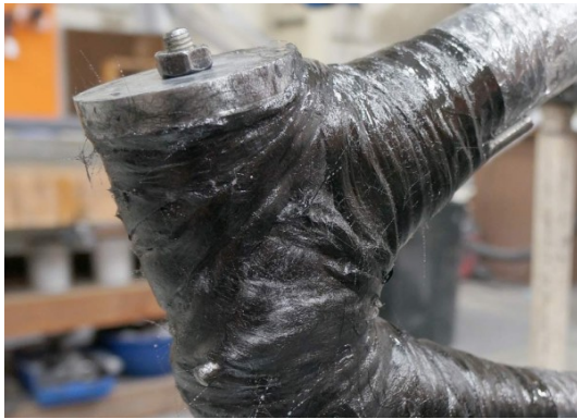
(a) A Junction of Carbon Fibre Tubes by Means of Carbon Fibre Tow e
