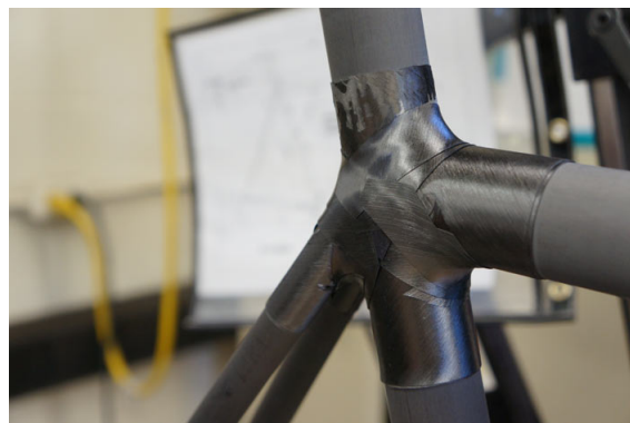
(b) A Junction of Carbon Fibre Tubes by Means of Carbon Fibre Sheets f
