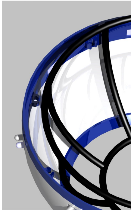
Figure 7.8: Shell Connection to Load Carrying Structure
