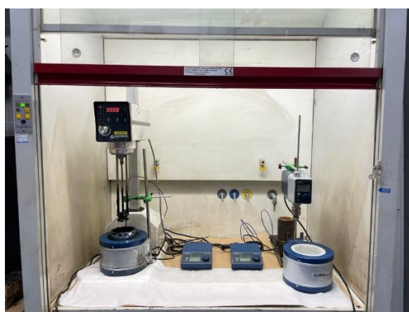
Fig. 2.5 High-speed shear machine, overhead stirrer and heating bath used for preparation
