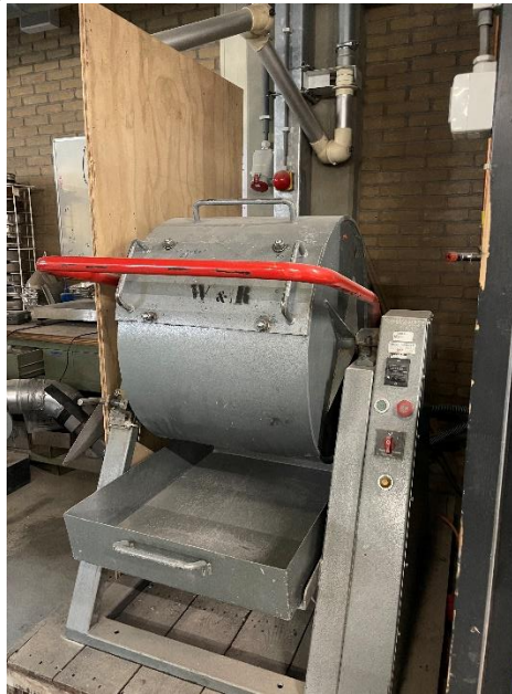
Fig. 2.9 Los Angeles Abrasion machine used in Cantabro test
