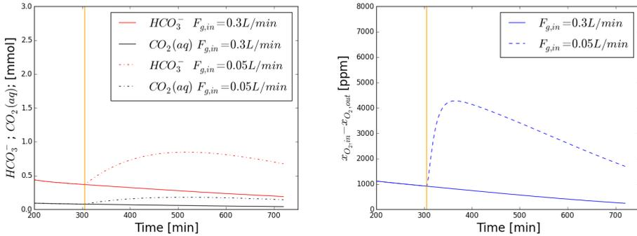
Figure 2.16: Simulation of the liquid  $CO_2$  and  $HCO_3^-$ , and the gas phase  $O_2$  profiles; with constant and adapted gas inflow rates. The orange line indicates where the flow rate is changed from 300 to 50 mL  $min^{-1}$ .
