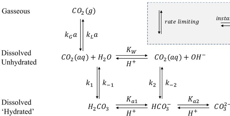
Figure 2.6: Reaction scheme of inorganic carbon in aqueous solution. Reactions that take place over the vertical axis are rate limiting, and reactions taking place over the horizontal axis are instantaneous protonation equilibria. In the gas-liquid exchange the  $k_G a$  and  $k_L a$  have the same physical meaning but are written from the perspective of the gas or liquid phase.
