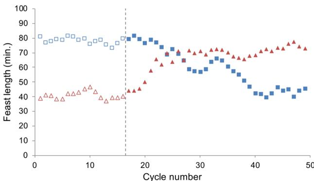
Figure 4.3: Change in feast length of  $\text{SBR}_{\text{HCl}}$  (red triangles) and  $\text{SBR}_{\text{H}_2\text{SO}_4}$  (blue squares) when switching their respective acids for pH control. Open figures represent the steady state feast length of fifteen cycles prior to the acid shift, the dashed line at cycle 16 indicates the moment where the acids were changed.
