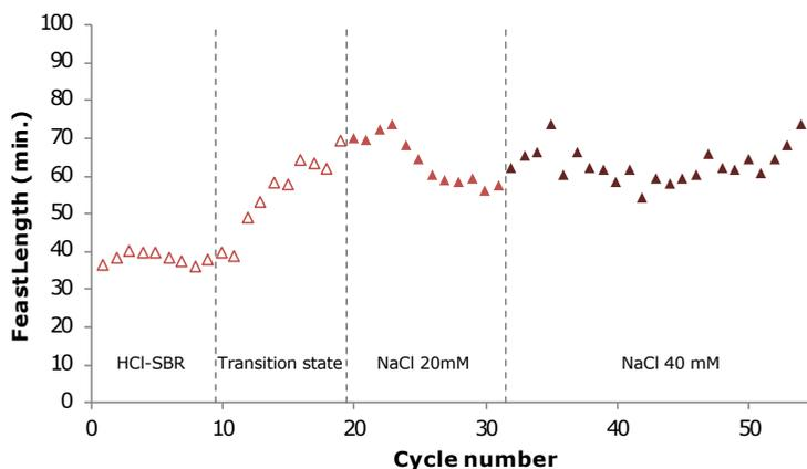
Figure 4.7: Feast length of  $SBR_{HCl \rightarrow H_2SO_4}$  after switching the acid to  $H_2SO_4$  (from cycle 10) during cultivation with increased NaCl (from cycle 20), 20mM in light triangles and 40mM in dark triangles. *P. acidivorans* remained the most abundant species in  $SBR_{HCl \rightarrow H_2SO_4}$  for 30 cycles with the NaCl supplemented medium, but eventually the community shifted towards a community dominated by *Zoogloea sp.* after 40 cycles (Figure 4.9).
