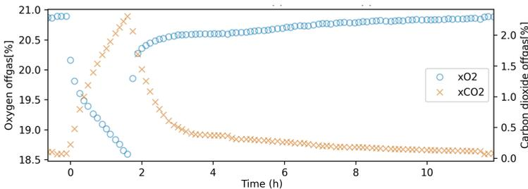
Figure 2.8: Example off-gas measurement of a single operational cycle. At  $t=0$  a substrate pulse is given, which around  $t=2$  h is completely consumed leading to a drop in respiration activity. The goal of the Particle Filter is to convert these measurements to the biological respiration rates.
