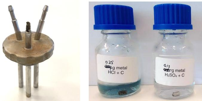
Figure 4.5: Photographs of an inlet triplet (left) of which the acid inlet is significantly corroded, and two acid bottles (right) with 5 mL 1 M HCl, and 5 mL 0.5 M  $\text{H}_2\text{SO}_4$  with a small piece of 316L reactor metal after 30 days.
