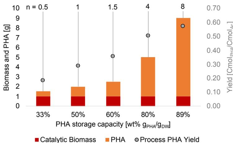
Figure 5.6: Visual representation of the difference in PHA production capacity when expressed as dry weight fraction. For each gram of catalytic biomass that is produced (red),  $n$  gram of PHA need to be produced (orange) to reach the PHA storage capacity as described on the x-axis. The grey circles denote the overall process yield, expressed as the amount of PHA that is produced from one Cmol of acetate substrate.
