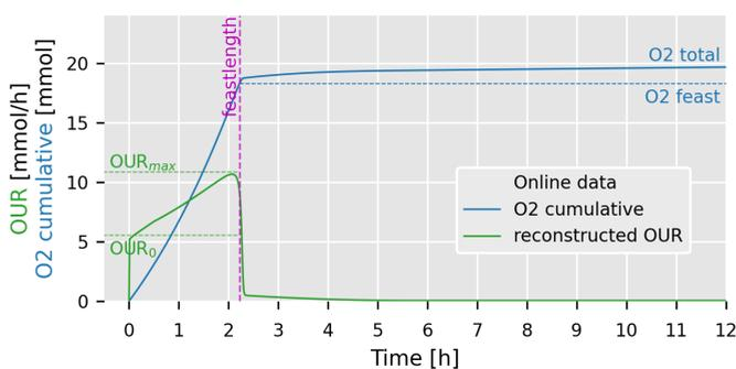
Figure 2.9: Schematic representation of how the reconstructed oxygen uptake rate (OUR in green) can be used to derive cycle specific key indicators. After the substrate pulse at  $t=0$ , a change in OUR is observed until the substrate is depleted at the end of the feast phase (feastlength in purple). By integrating the OUR over the cycle (O2 cumulative in blue), it is possible to estimate the fraction of total oxygen that is consumed during the feast phase.
