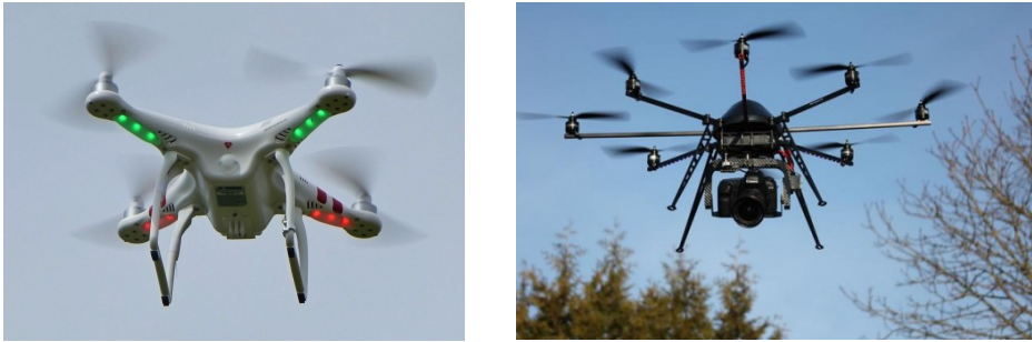
Figure 1.1: Photos of two types of multi-rotor drones. a.) Quadrotor b.) Octorotor.
