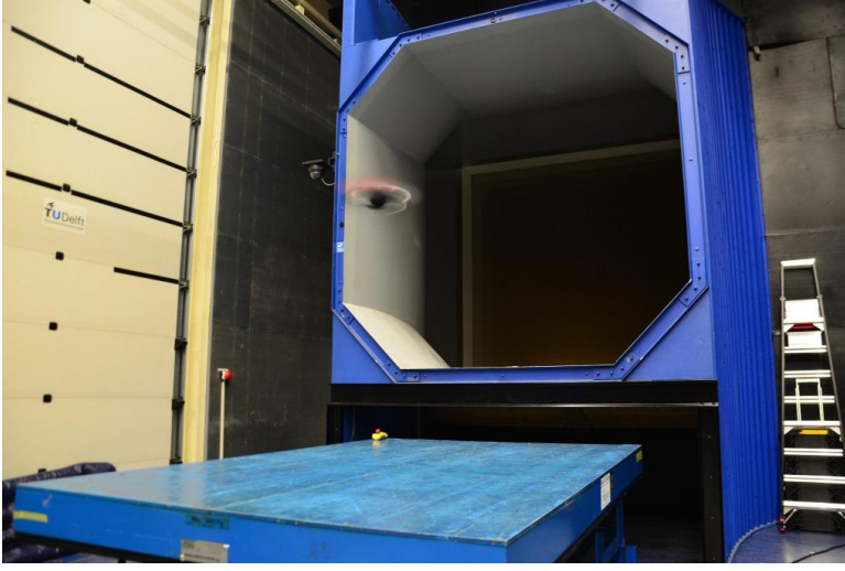
Figure 4.1: Figure of Open Jet Facility and the spinning quadrotor during flight.
