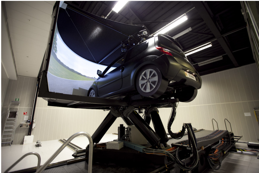
Figure 2.4: Renault ULTIMATE driving simulator. Used in Colombet et al. (2018), image source: VSimulation (2020).
