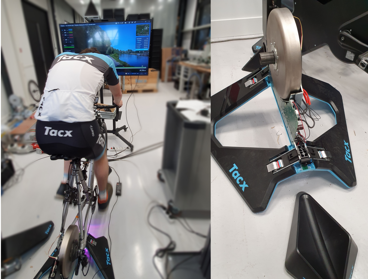
Figure 3.4: Simulator setup to be used for fixed bicycle simulator experiments. Visible are the same bicycle as in outdoor experiments, the simulator, and the visual representation of an outdoor cycling environment, on the left. On the right, the setup without a mounted bicycle is visible.
