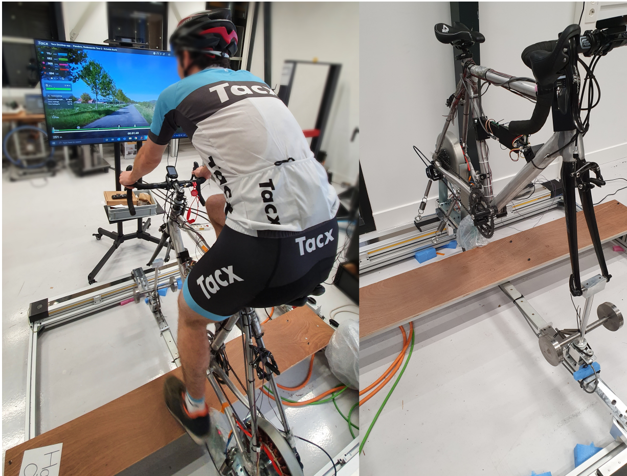
Figure 3.3: Simulator setup to be used for bicycle simulator experiments. Visible are the same bicycle as in outdoor experiments, the simulator, and the visual representation of an outdoor cycling environment. On the left, with a participant, on the right, a front view.
