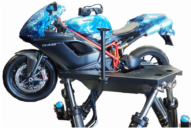
Figure 2.6: Cruden Motorcycle Simulator, as used in Westerhof (2017)
