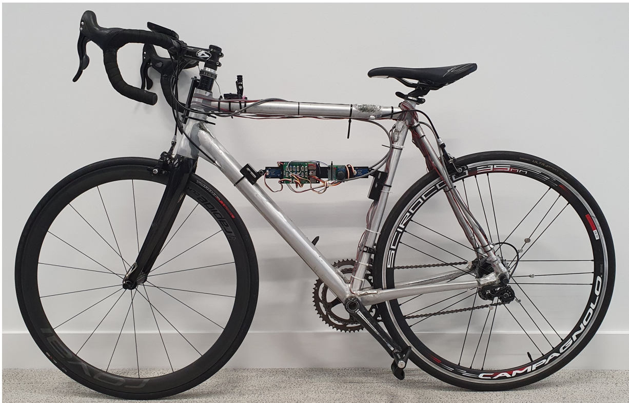
Figure 3.2: Measurement bicycle with measurement board (see Appendix A) attached to its frame. Remnants of previous studies are still present in the form of strain gauges and wires, which could not be removed.
