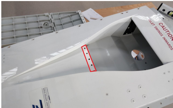
Figure 3.2: Isometric view of the NACA ram-air inlet of the Airbus A320 with the location of the 'axis of rotation' indicated by the red box.
