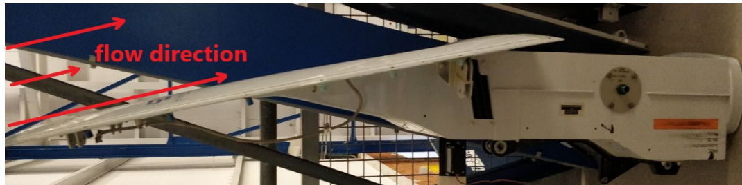
Figure 3.1: Side view of the NACA ram-air inlet of the Airbus A320. The flow direction is indicated with red arrows.
