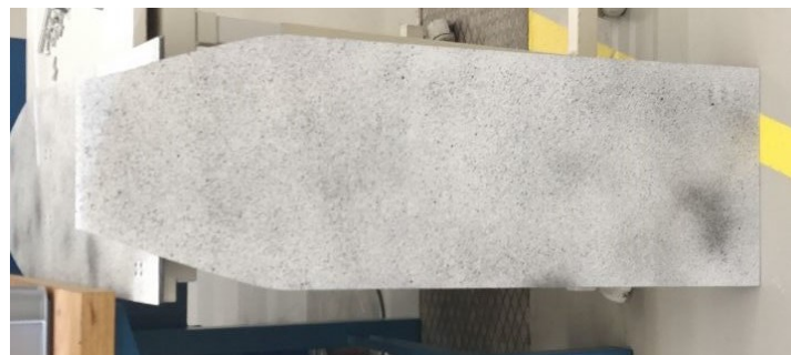
Figure 3.9: Morphing (laminite) flap. The morphing flap is attached with countersunk bolts to the NACA ram-air inlet at the 'axis of rotation'
