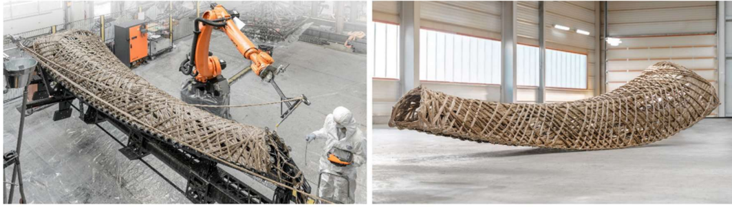
Figure 18: LivMats pavilion fabrication setup (left) and component after curing (right) livMatS Pavilion / ICD/ITKE University of Stuttgart (2022, 14 Aug). ArchDaily. Accessed 10 Dec 2023. < https://www.archdaily.com/966168/livmats-pavilion-icd-itke-university-of-stuttgart > ISSN 0719-8884
