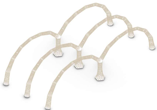
Double Barrel with support columns Steinfort, R.T. (2024)
