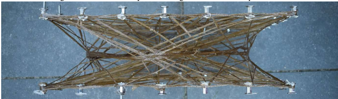
Figure 54: Top view of the edging of the frames, showcasing the winding pins to be more integrated into a bundle of points Steinfort, R.T. (2024)
