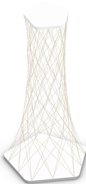
Fibrous column Steinfort, R.T. (2024)
