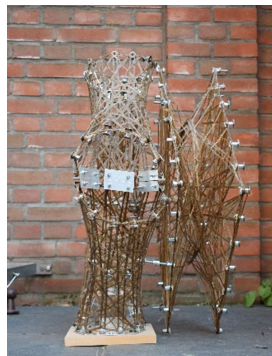
Figure 56: The different panel compositions in the structural fragment (from left to right: panel 1, 2, 3 and 4) Steinfort, R.T. (2024)
