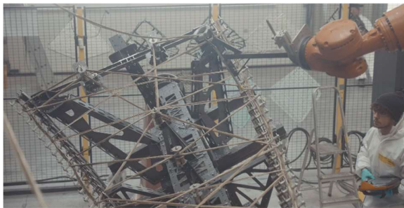
Figure 17: Winding of the flax fibrous LivMatS Pavilion beam element and the winding syntaxes livMatS Pavilion / ICD/ITKE University of Stuttgart (2022, 14 Aug). ArchDaily. Accessed 10 Dec 2023. < https://www.archdaily.com/966168/livmats-pavilion-icd-itke-university-of-stuttgart > ISSN 0719-8884
