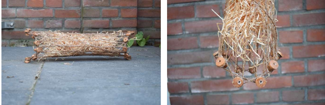
Figure 48: Beam with an alternative (biobased) material, wood, for the winding pins Steinfort, R.T. (2024)
