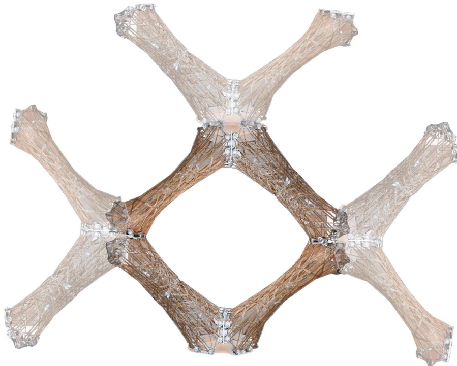
Figure 47: Repetition of the structural fragment to form the overall assembly Steinfort, R.T. (2024)
