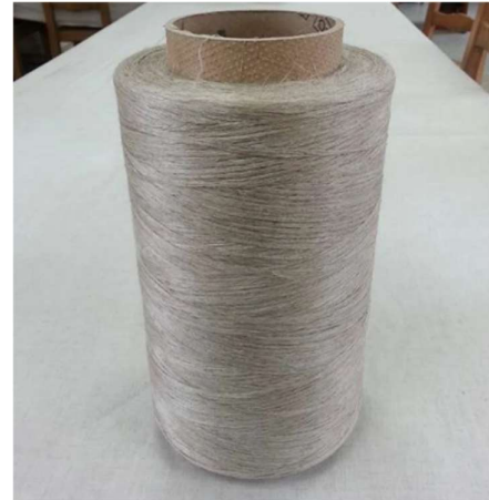
Figure 35: 2.5 kg Depestele Flax reel approx. 5km (Circular-Structures, 2023)
