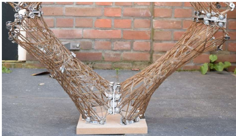
Figure 42: Different amounts of fiber-to-fiber interaction showcased on the left with beam 3 (more fiber-to-fiber interaction) and on the right beam 1 (less fiber-to-fiber interaction) Steinfors, R.T. (2024)
