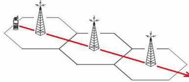
Figure 3.6: Cell structure of cellular networks. [source: [5]]
