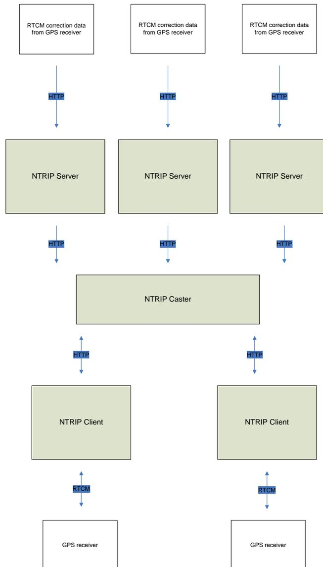
Figure 4.1: Generic NTRIP set up.
