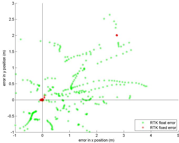
Figure 5.18: Demonstration of incorrect RTK ambiguity fix.
