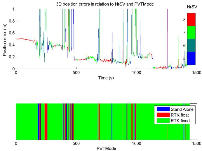
Figure 5.31: Septentrio error to ground truth in relation to the PVT Mode.
