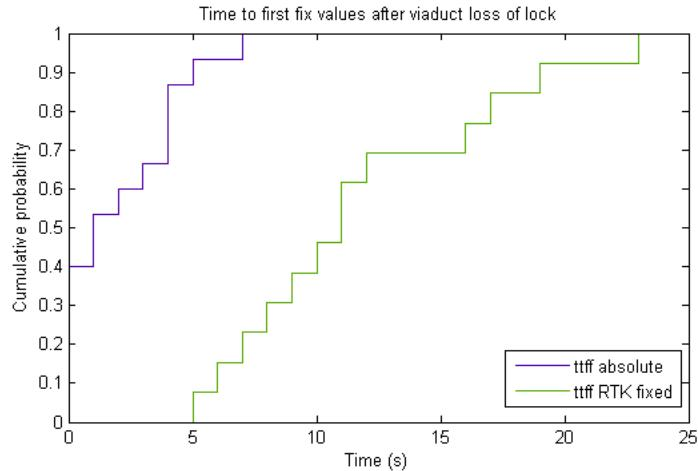
Figure 5.40: Cumulative time to first fix probabilities, absolute and RTK fixed.
