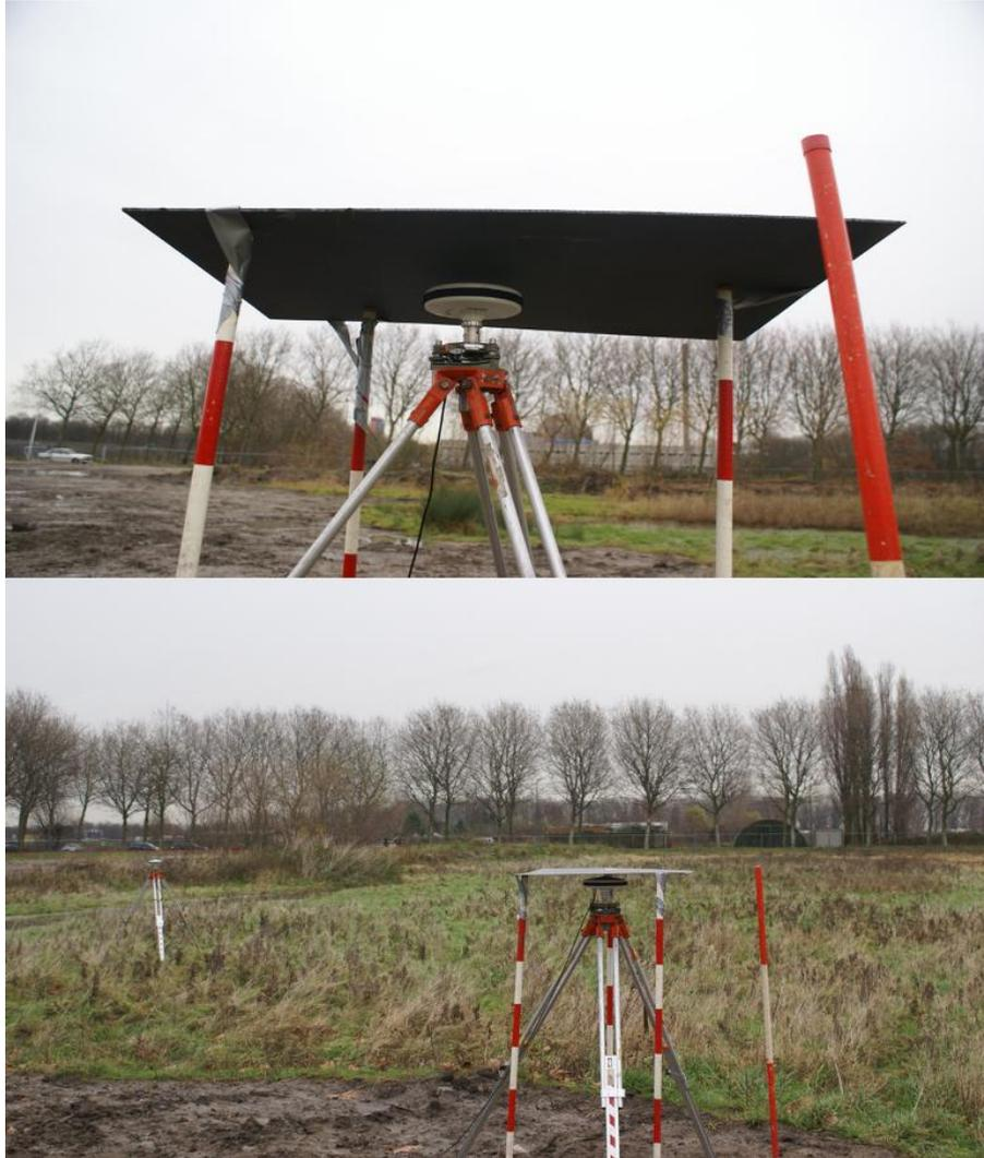
Figure 5.5: Rover antenna covered with carbon fibre material, supported by the wooden construction.
