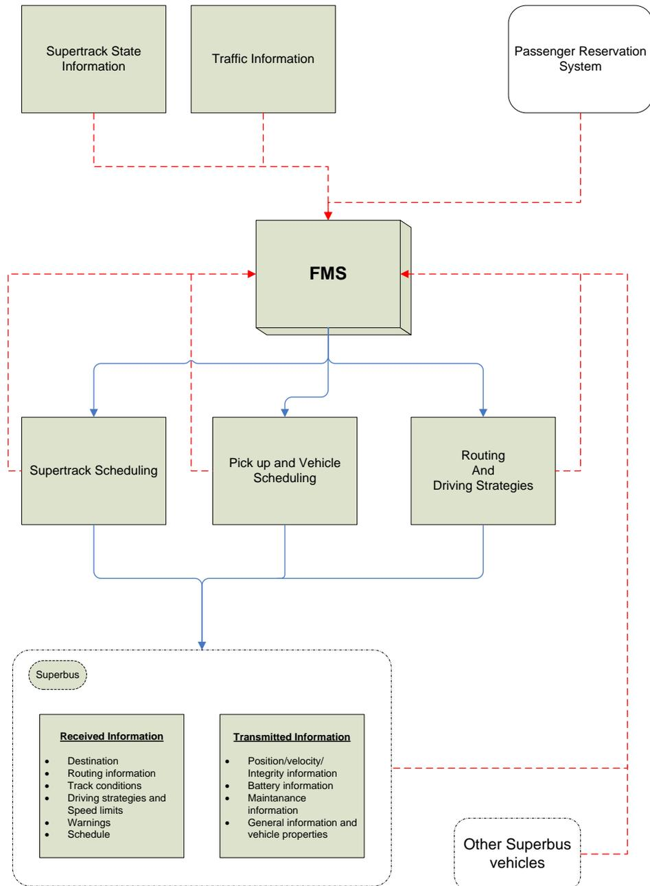
Figure 4.8: Superbus FMS example.
