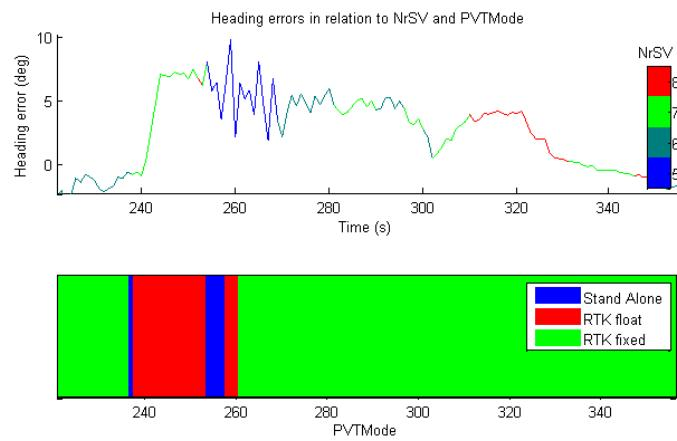
Figure 5.35: Heading error detail, showing dependence to the NrSV.
