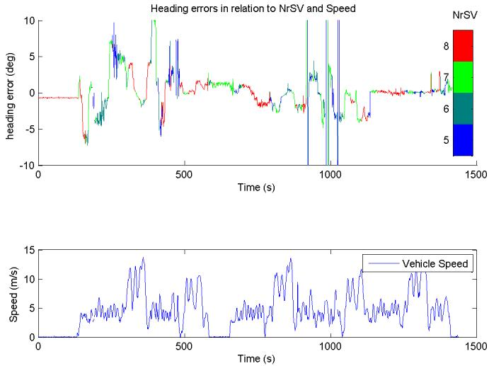
Figure 5.34: Heading error in relation to the NrSV and Velocity.
