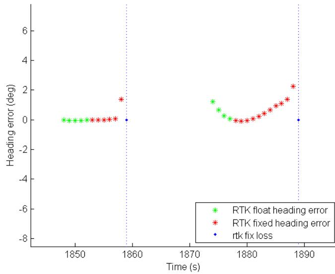
Figure 5.20: Detail: Divergent heading error before loss of RTK.
