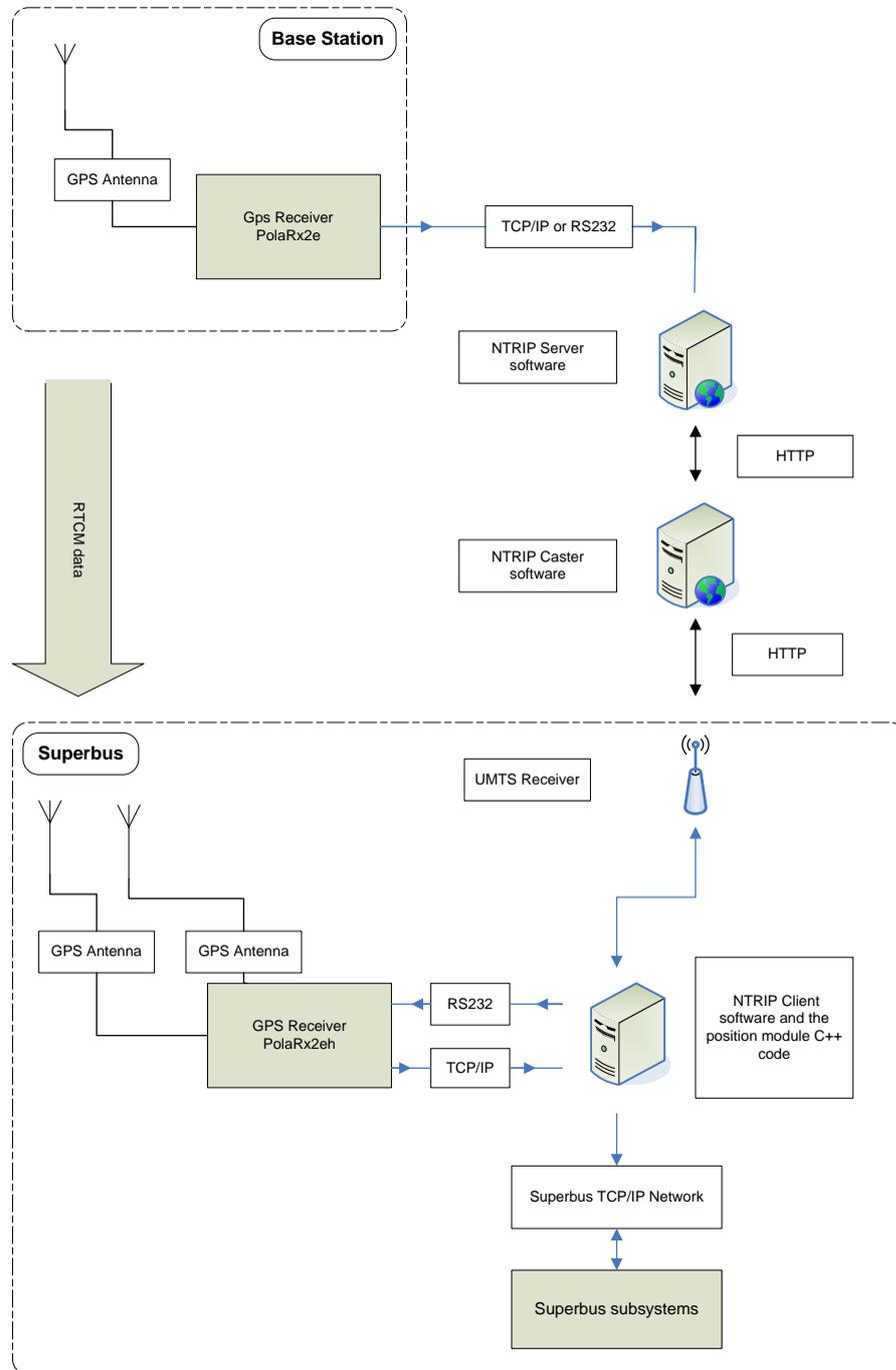
Figure 4.2: Superbus GPS system lay out with dedicated base station.
