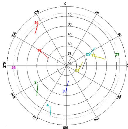
Figure 5.38: Skyplot over Delft, during the A4 experiment.
