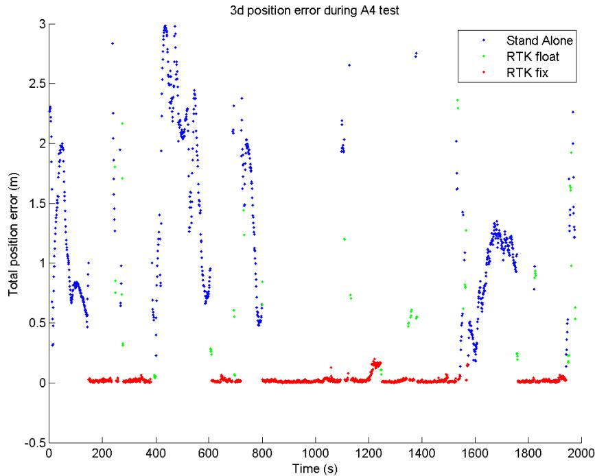
Figure 5.39: Total Position error during A4 with respect to PVT Mode.
