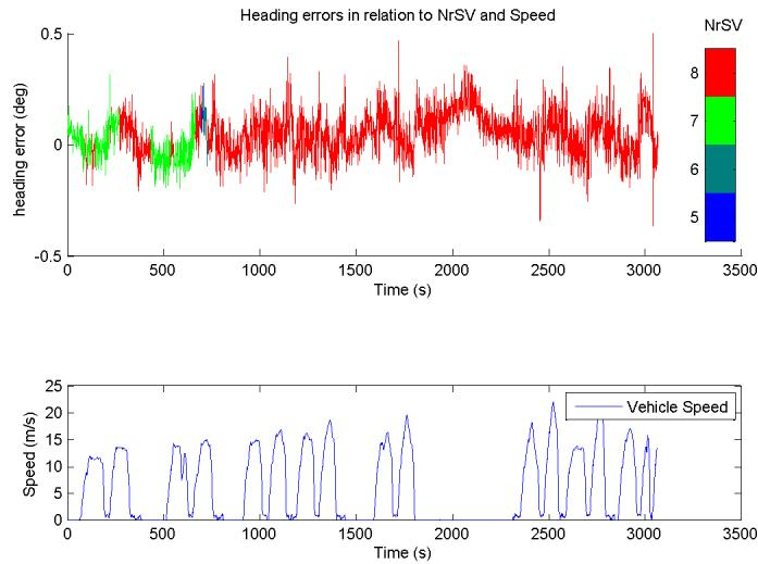
Figure 5.28: Septentrio speed in relation to heading errors.
