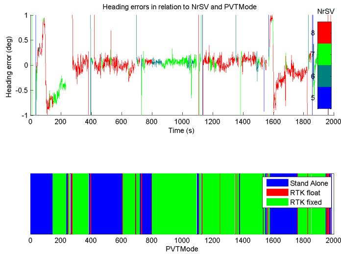
Figure 5.41: Heading errors versus PVT Mode and Number of satellites in view.
