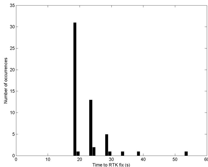
Figure 5.21: Histogram of the reacquisition times. A total of 56 trials
