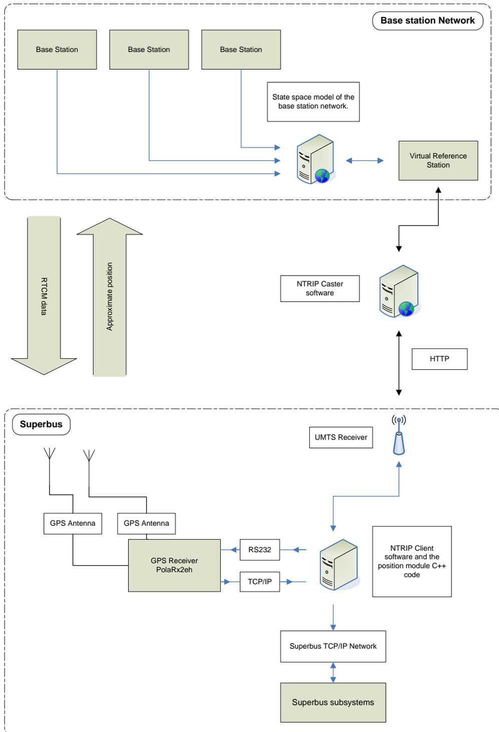
Figure 4.3: Superbus GPS system lay out with network based VRS.
