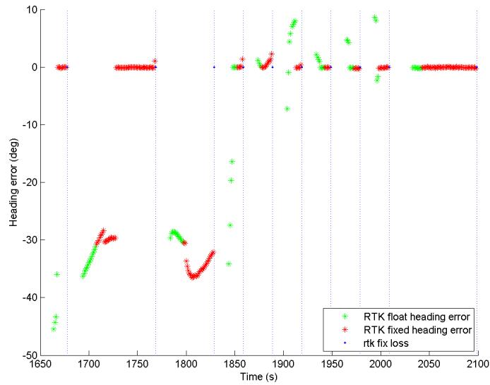
Figure 5.19: Heading error due to unfixed secondary antenna.
