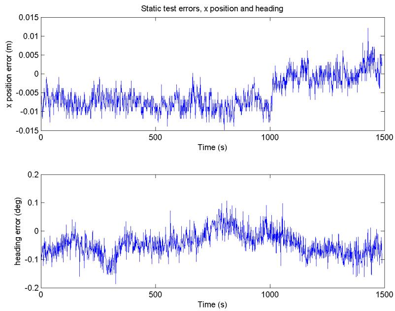
Figure 5.15: X position and heading error over time.
