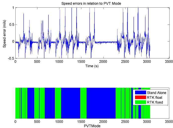
Figure 5.27: Receiver speed comparison of the Duifpolder experiment.
