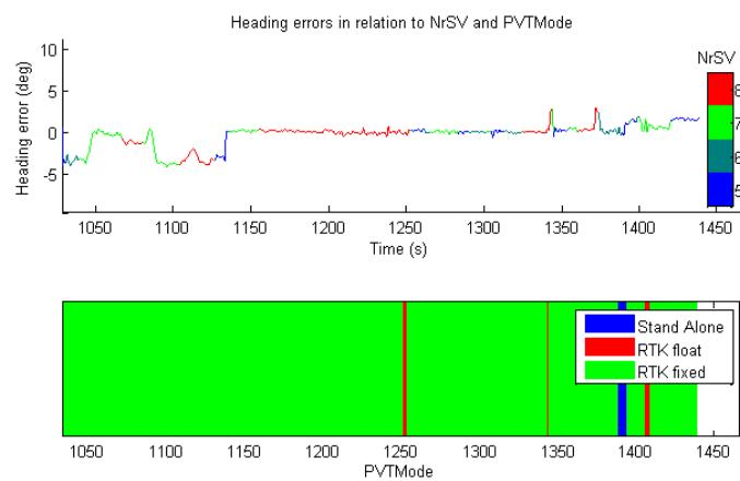
Figure 5.36: Heading error detail, showing dependence to the NrSV.
