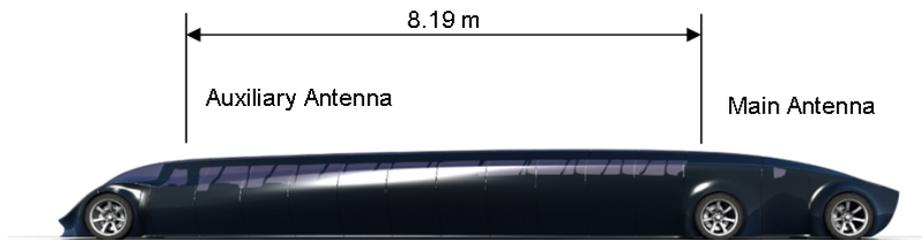
Figure 4.5: Placement of the two GPS antennas in the Superbus.
