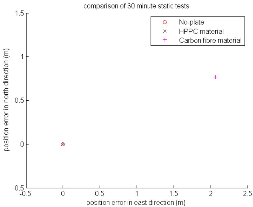
Figure 5.11: Comparison of three, 30 minute, static solutions.
