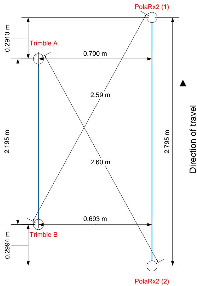
Figure 5.8: Vehicle frame overview, dimensions and antenna placement. Vehicle front is top of figure.
