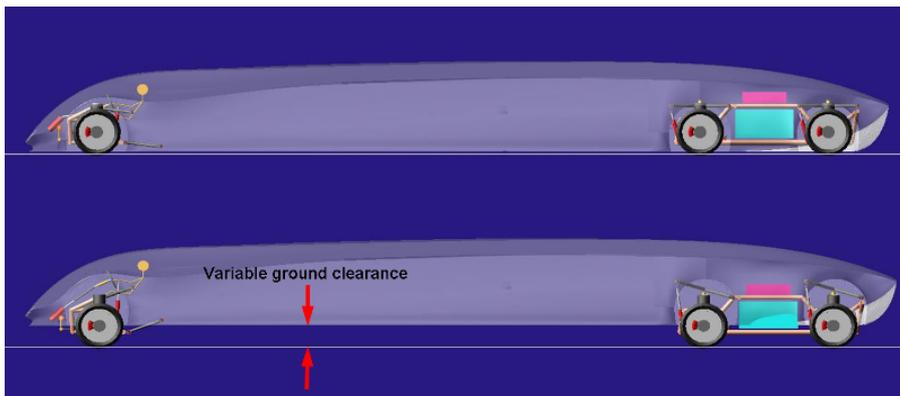
Figure 2.4: Ground clearance in high and low settings. [source: Superbus]
