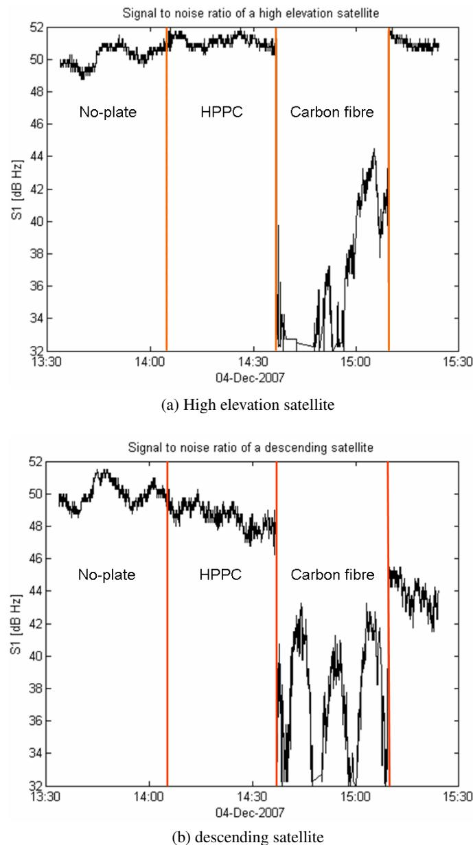
Figure 5.13:  $C/N_0$  (signal strength) ratios of two satellites under three circumstances.
