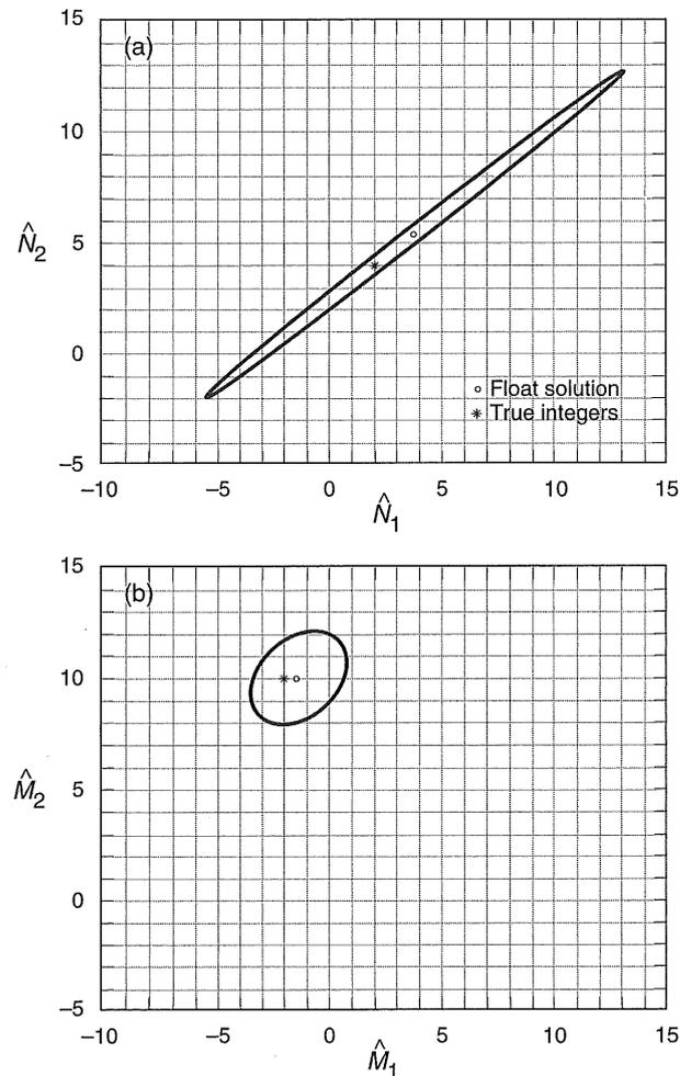
Figure 3.5: 2D example constant cost ellipsoids before (a) and after (b) the decorrelation step. Rounding in the first scenario would produce incorrect integers of  $(4, 5)$ , while rounding in the second scenario produces the correct  $(-2, 10)$ . [Source: [31]]
