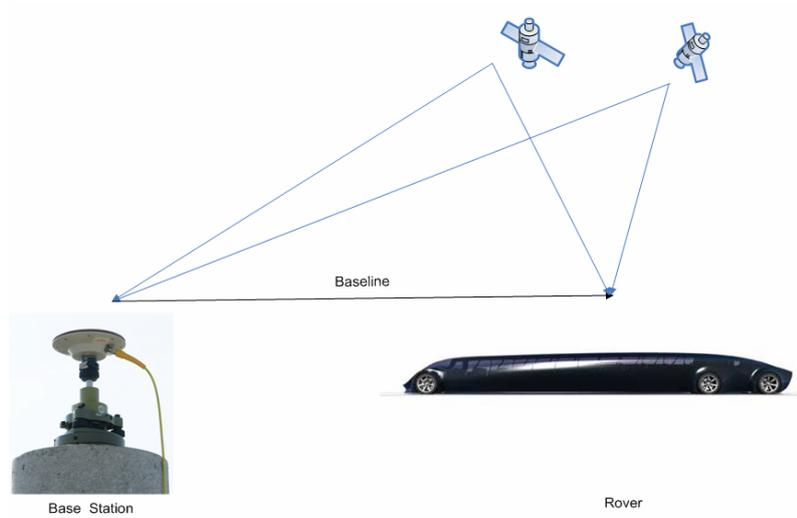
Figure 3.3: Graphical representation of an RTK set up.
