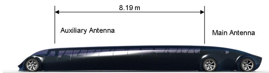
Figure 4.5: Placement of the two GPS antennas in the Superbus.
