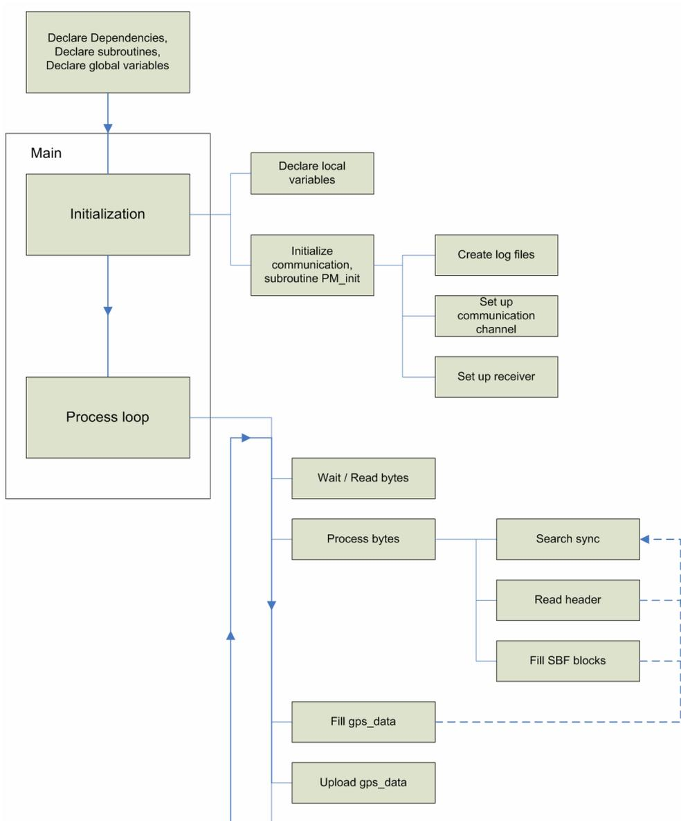
Figure 4.6: Position Module, high level lay out.
