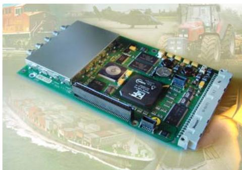
PolaRx2eH can be connected to 2 dual-frequency antennas whereas PolaRx2e@ can be connected to up to 3 antennas, of which the main antenna can be dual-frequency while the auxiliary antennas are single-frequency. Both receiver types have 48 hardware channels, which can be flexibly assigned to track satellites in single or dual-frequency on 1, 2 or 3 antennas in parallel (i.e. without antenna multiplexing).
