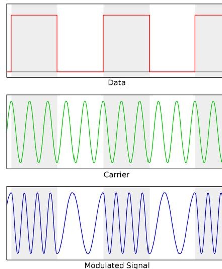
Figure 3.7: Representation of frequency shift modulation. [source: wikipedia]
