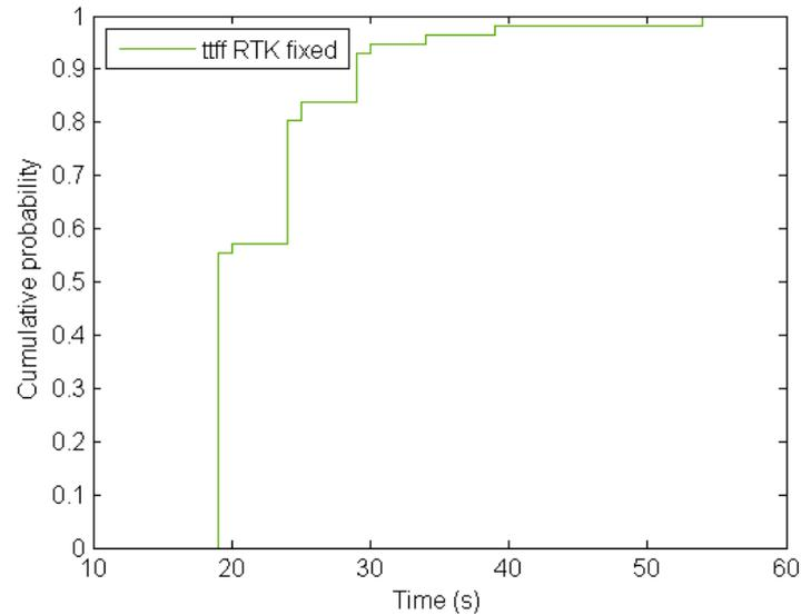
Figure 5.22: Cumulative representation of reacquisition times.
