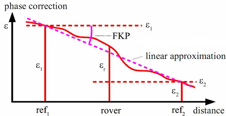
Figure 3.4: Graphical representation of relative positioning errors. [Source: 06-GPS]
