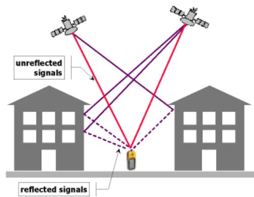
Figure 3.2: Graphical representation of a multipath situation. [source: BKG]
