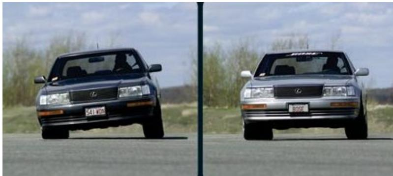
Figure 4.7: Vehicle behaviour during cornering. Active suspension is enabled on the right. [source: Bose]
