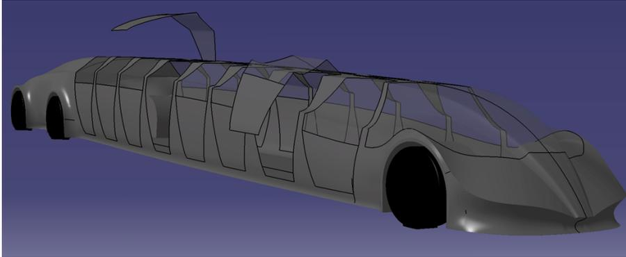
Figure 2.3: Gull-wing door design. [source: Superbus]
