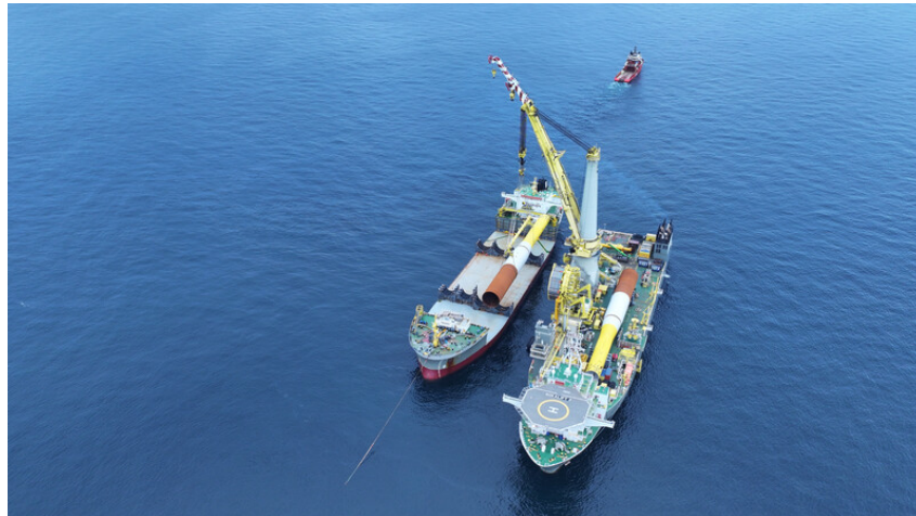
Figure 2: Feeder operation during monopile installation: the Bokalift 2 lifts monopiles from a feeder barge.
