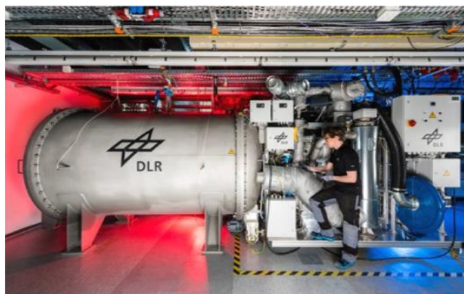
Figure 13: Picture of the hybrid SOFC-MGT emulator at DLR
