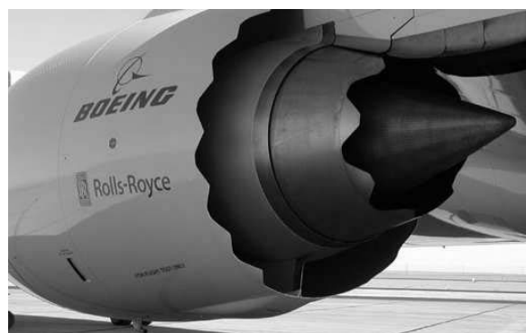
Figure 2.8: Turbofan engine (Trent 800) with nacelle design to improve the mixing process between the exhaust and ambient air. Part of the joint Boeing/Rolls Royce Quiet Technology Demonstrator program. [www.rolls-royce.com]
