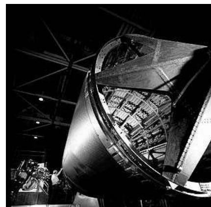
Figure 1.15: Production of one-piece fuselage parts for the Boeing 787 made of Carbon fiber reinforced plastic. [www.boeing.com]
