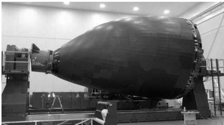
Figure 1.15: Production of one-piece fuselage parts for the Boeing 787 made of Carbon fiber reinforced plastic. [www.boeing.com]
