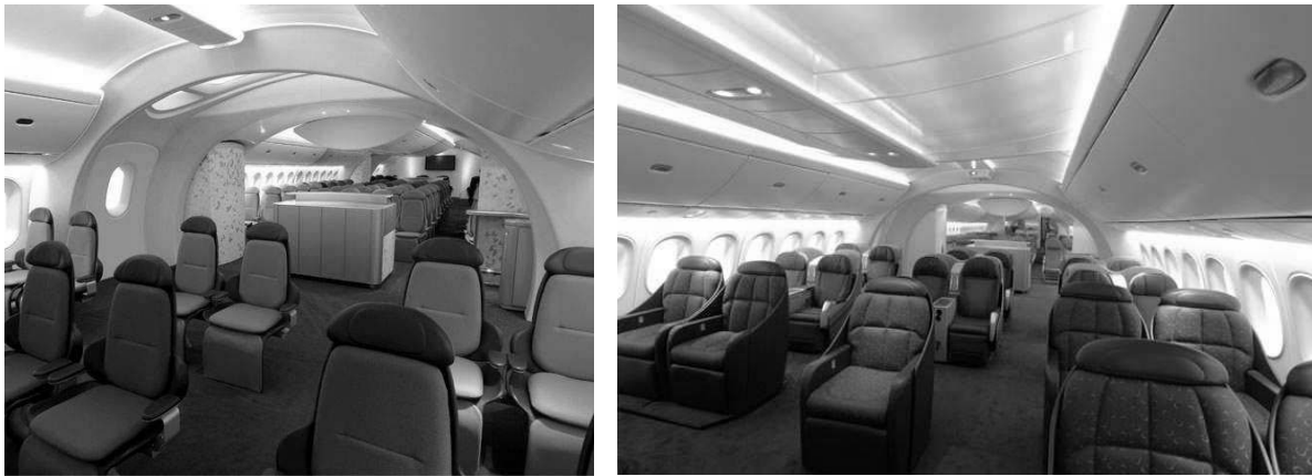
Figure 1.16: The Boeing 787, which will have a full composite fuselage. The application of CFRP opens new possibilities like larger windows. [www.boeing.com]
