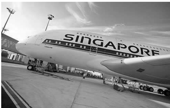
Figure 1.12: Singapore Airlines Airbus A380 March 2008 together with an impression of the economy class interior. The fuselage partially made out of GLARE, which is a laminated material made out of aluminium and glass fiber layers. [ www.hemmy.net ]
