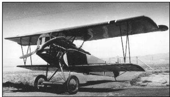
Figure 1.2: Fokker D.VII (January, 1918); Steel framework fuselage covered with fabric. [ www.aviation-history.com ]
