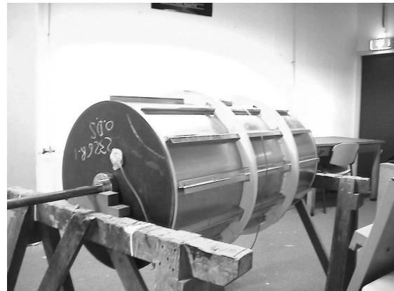
Figure 8.29: Test set-up of the cylinder with 12 stringers and 2 frames.
