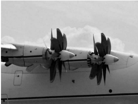
Figure 2.6: D-27 Turboprop engine with counter rotating swept blades on an An-70. [www.wikimedia.org]
