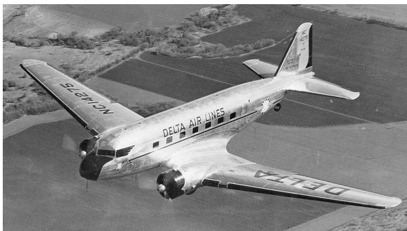
Figure1.4: DC-2; Example of a first generation aircraft with an aluminium stiffened skin fuselage. [ www.stinsonflyer.com ]
