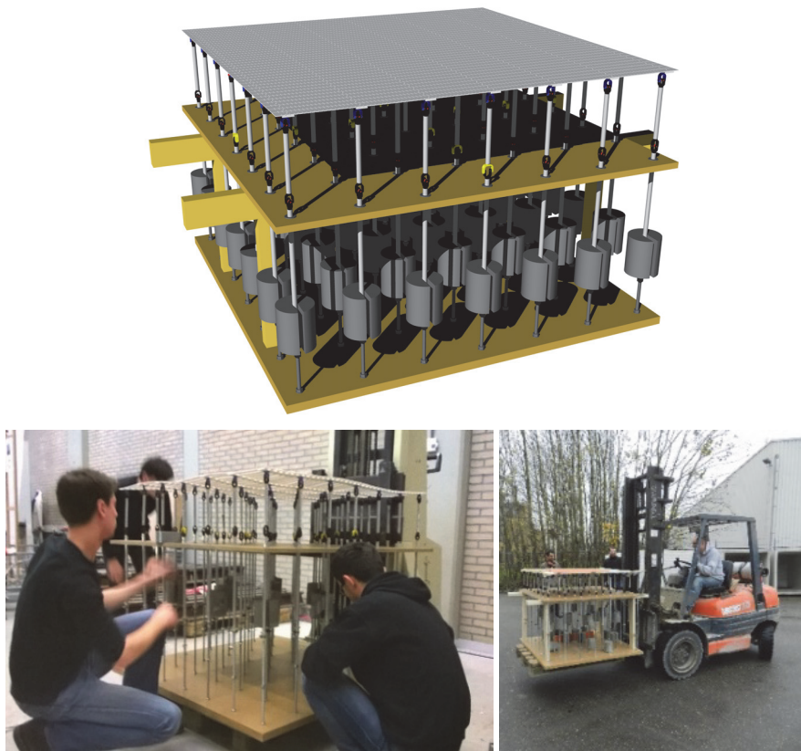
Figure 5: Drafting, assembly and transport to the concrete product factory of the semi-full-scale prototype of the Kine-mould
