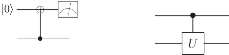
Figure 1.2: Left: Circuit including a single CNOT and a measurement of the top qubit. The black dot represents the control qubit, the  $\oplus$  the target qubit. Right: Circuit including a single controlled- $U$ . The black dot represents the control qubit, the square with  $U$  the action of applying  $U$  to the target qubit.
