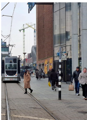
Lay-out and dimensions: Narrow sidewalk next to the tram line force pedestrians to sidestep, often causes collisions.
