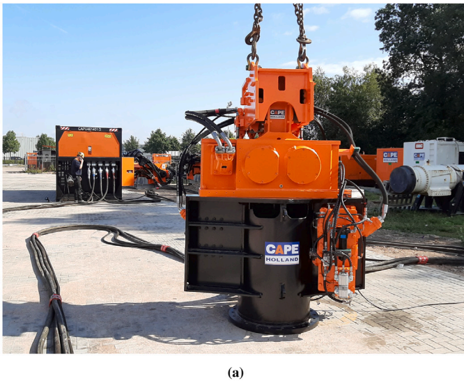
Fig. 1. The GDP shaker: (a) view at the manufacturing site; (b) shaker connected to a test pile via a bolted flange connection.
