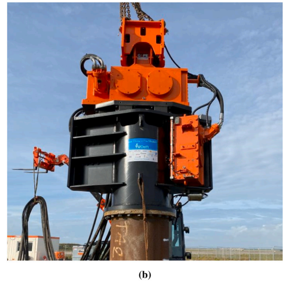
Fig. 1. The GDP shaker: (a) view at the manufacturing site; (b) shaker connected to a test pile via a bolted flange connection.
