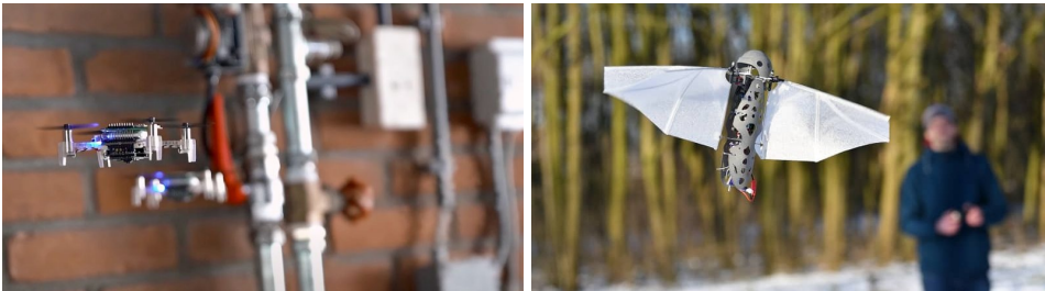
Figure 1.1: Small drones can operate in high-risk scenarios. A group of tiny quadrotors ( left ) collaborating to find a gas source [10]. Flapping wing drones ( right ) can safely operate around humans.
