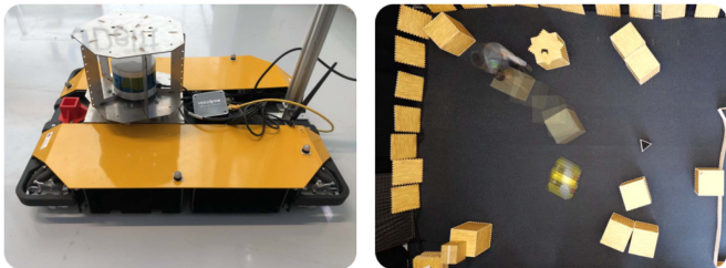
Fig. 5. Real ground robot used to run the experiments. For the real-world experiment, we used a Clearpath Dingo with a Velodyne VLP16 mounted on top (left). The real-world experiment shows the Dingo navigating through an environment where a human throws in obstacles (right).
