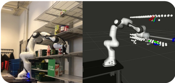
Fig. 13. Real robotic manipulator used to run the experiments. A Franka Emika Panda is confronted with an unknown shelf environment in a supermarket. Arrows indicate the normals of the planes obtained by the FSD. Different colors indicate different links on the robotic arm. .
