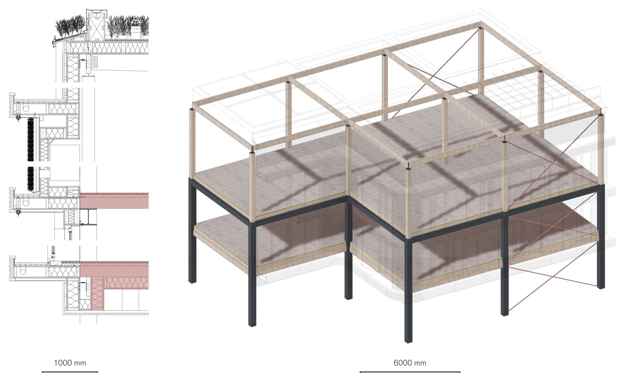
Secondary Structure & Bracing
