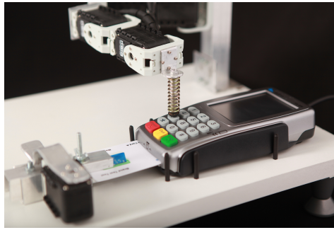
Figure 2.4: Photo of an early version of the test robot while testing a PED.
