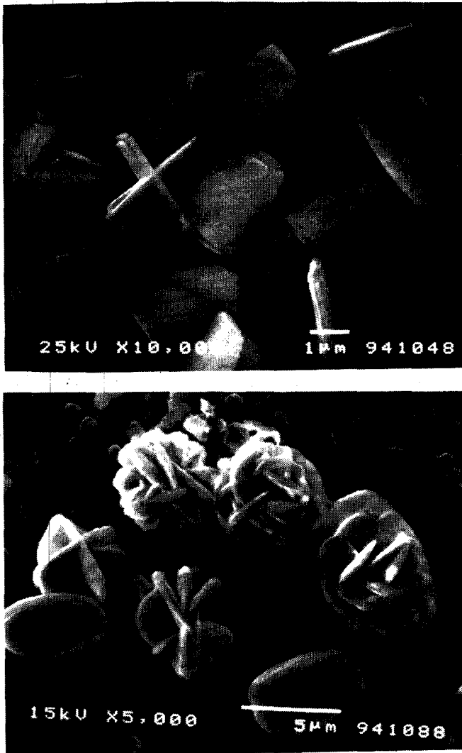
Fig. 7.7. SEM photograph of the crystals which have been filtered with a 0.45 \mu\text{m} membrane filter, about 1 hour after the start of the reaction. On the upper photograph, the PMA-PVS concentration was 0.02 ppm and on the lower one 0.04 ppm. For both, the starting supersaturation was 24.5. The particles with no or very small amounts of PMA-PVS have the form of platelets.
