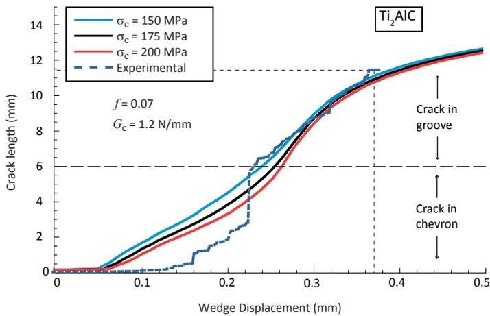
Figure 3.8: Crack length as a function of wedge displacement for three distinct values of the fracture strength and for a fixed fracture energy of  $0.725 \text{ Nmm}^{-1}$  for the  $\text{Ti}_3\text{SiC}_2$  and  $\text{Ti}_2\text{AlC}$  samples.
