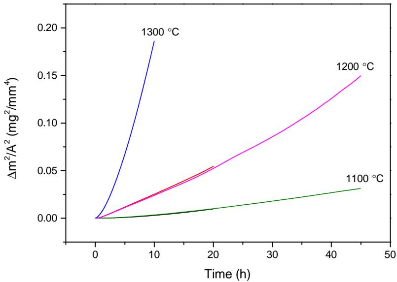
Figure 5.5: (a) Weight gain and calculated scale thickness for an oxide comprised of  $\text{SiO}_2:\text{TiO}_2 = 1:3$  and (b) square or the normalized weight gain for isothermal oxidation in synthetic air for 10 to 20 h at 1100, 1200 and 1300 °C.
