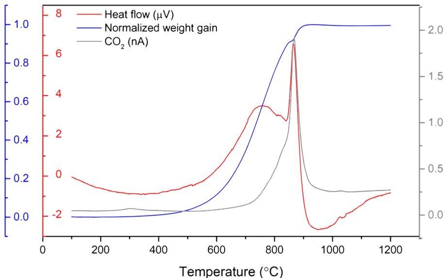
Figure 6.7: Heat flow, mass gain (TG) and CO<sub>2</sub> signal of Ta<sub>2</sub>AlC powder heated up to 1200 °C with 5 °Cmin<sup>-1</sup>.
