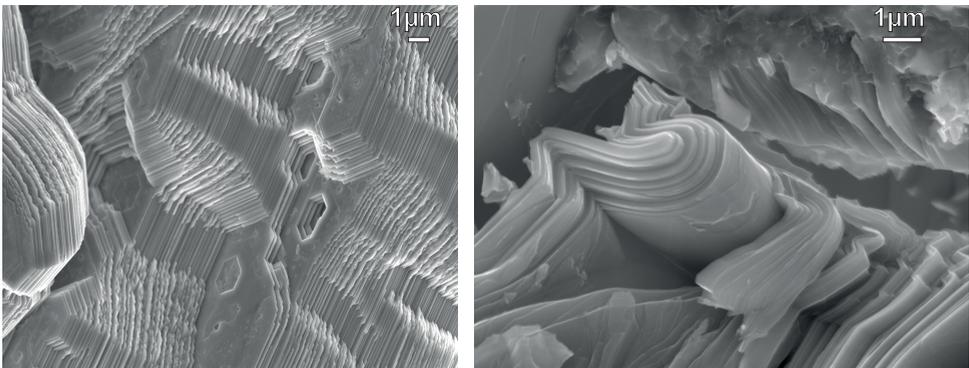
Figure 1.3: SEM images of lamellar structure and kinking.
