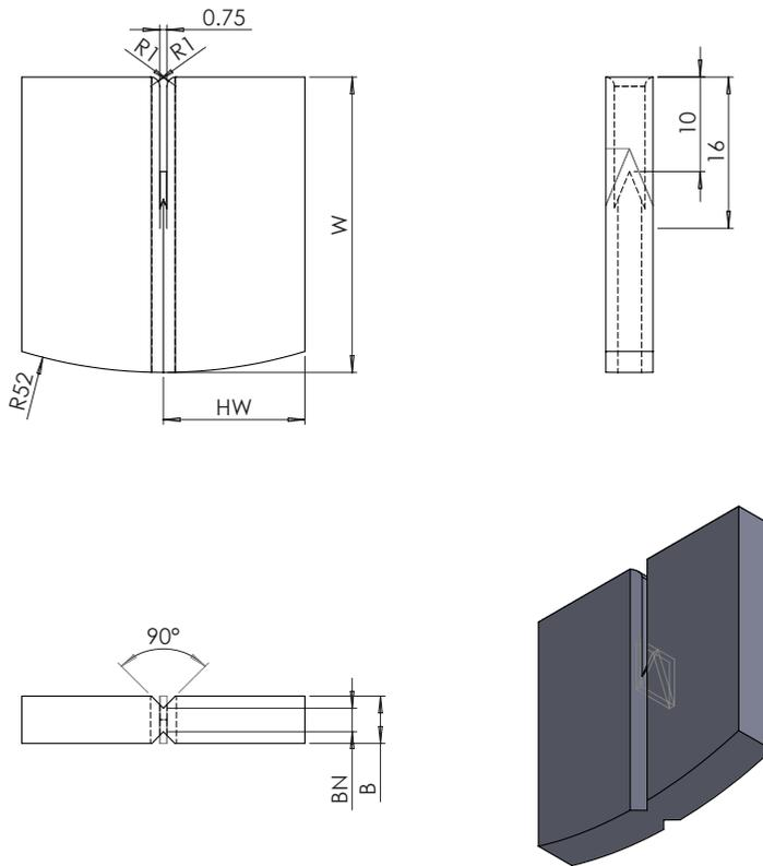
Figure 3.1: Wedge splitting test specimen geometry with lengths in mm.
