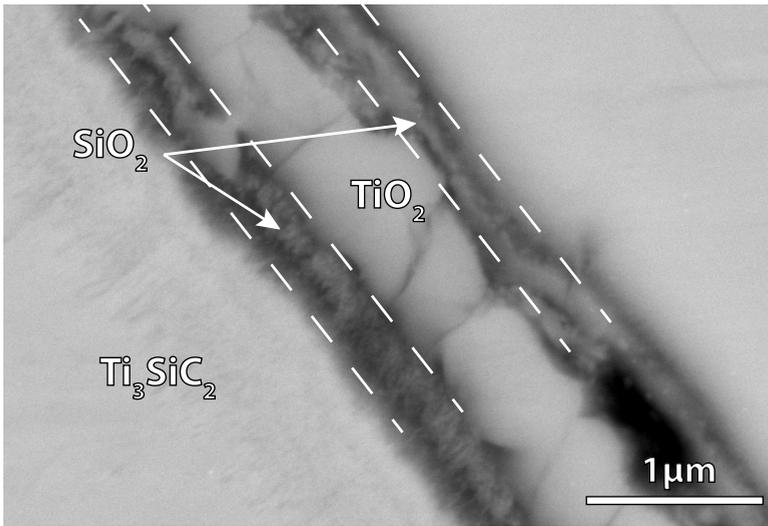
Figure 5.7: Crack in Ti<sub>3</sub>SiC<sub>2</sub> after oxidation at 1300 °C for 1 h. Local compositions as identified by SEM-XMA are indicated.
