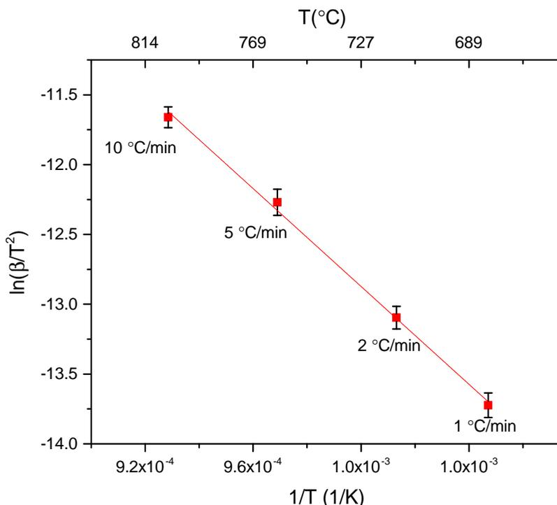
Figure 6.8: Kissinger points and linear fit of 1st reaction from DTA data on Ta<sub>2</sub>AlC heated with 1, 2, 5 and 10 °Cmin<sup>-1</sup>.
