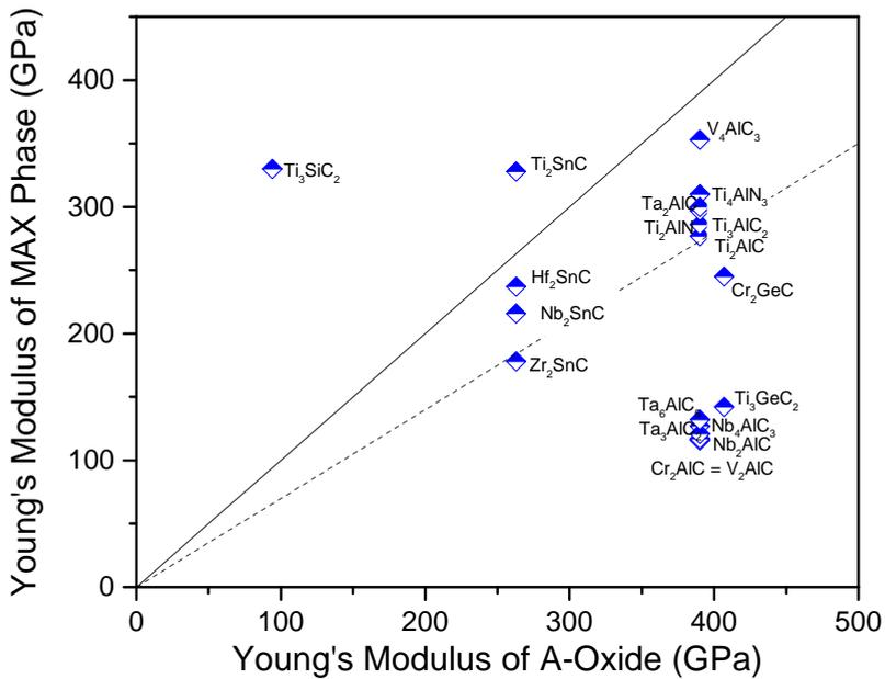
Figure 2.8: Young's Moduli of MAX phases and their respective A-element oxides. Upon loading negligible stresses in oxide if:  $E_{MAX} > E_{oxide}$  (see straight line). Significant stresses can arise when  $E_{oxide}$  is more than 30% larger than  $E_{MAX}$ ; see dotted line.
