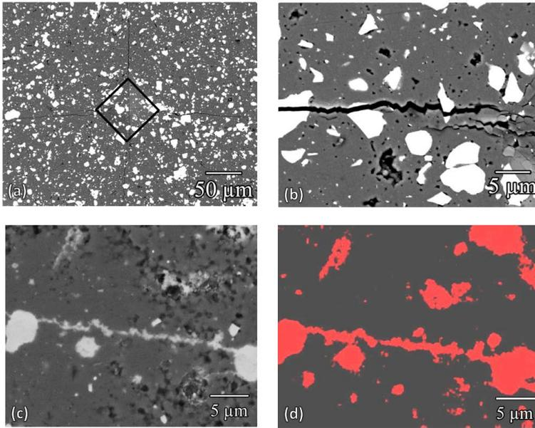
Figure 7.5: SEM micrographs of Al<sub>2</sub>O<sub>3</sub>/TiC composite. (a) Cracks created by Vickers indentation: (b) close-up showing crack-particle interaction, (c) healed crack after exposure to combustion environment for 4 h, (d) Ti X-ray mapping showing the filling of the healed crack.
