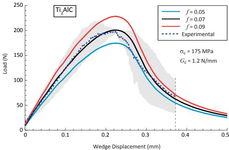
Figure 3.5: Wedge load as a function of wedge displacement for three distinct values of the coefficient of friction between the wedge and the  $\text{Ti}_3\text{SiC}_2$  and  $\text{Ti}_2\text{AlC}$  specimens. In accordance with the geometry shown in Figure 3.3, higher coefficients of friction effectively provide stiffer initial responses.
