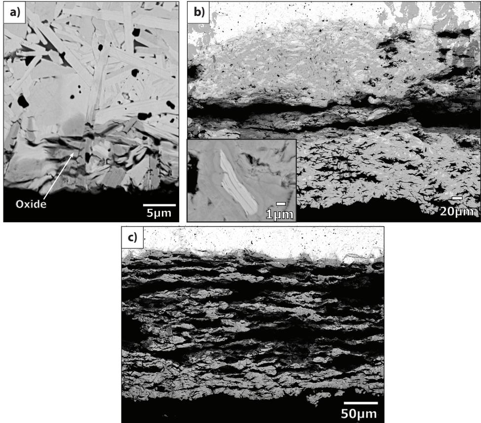
Figure 6.6: SEM images of oxide scales after 10 hours of isothermal oxidation of Ta<sub>2</sub>AlC in artificial air at a) 600, b) 700 and c) 800°C
