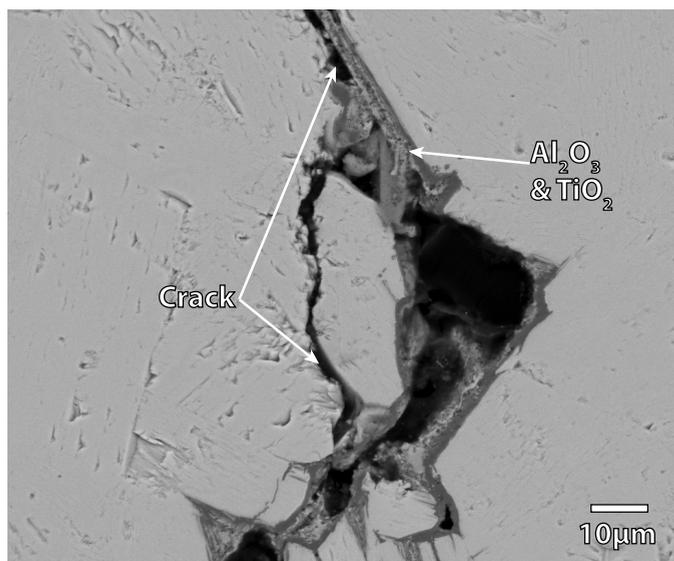
Figure 4.5: SEM backscattered electron image of cross-sectioned Ti<sub>2</sub>AlC sample cracked 3 times with two intermediate healing treatments. The final induced crack runs through the previously formed TiO<sub>2</sub> and Al<sub>2</sub>O<sub>3</sub>, as indicated.
