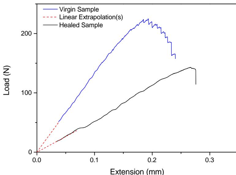
Figure 6.2: Load versus displacement curves of wedge loaded chevron notched  $\text{Ta}_2\text{AlC}$  specimen before and after isothermal oxidation at  $600^\circ\text{C}$  for 16 h in air. Samples were pre-loaded to approx. 20 and 55 N, thus both curves were extrapolated for better comparison.
