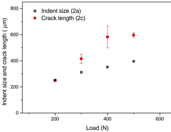
Figure 7.1: Vickers Indent size and crack length versus applied load of (a) Al<sub>2</sub>O<sub>3</sub> with 20 vol. % TiC composite and (b) fine grained Cr<sub>2</sub>AlC.
