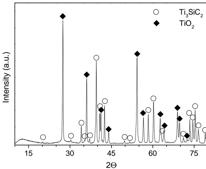
Figure 5.3: XRD pattern of  $\text{Ti}_3\text{SiC}_2$  after oxidation at  $1100^\circ\text{C}$  for 20 h.
