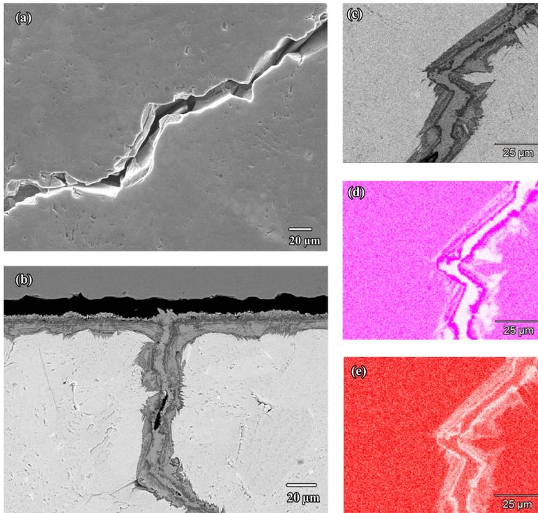
Figure 7.6: (a) Cracks in  $Ti_2AlC-A$  after quenching in water from  $850\text{ }^\circ C$ ; (b) cross-section of healed crack after exposure to combustion conditions for 4 h; (c) close up of healed crack; (d) Al X-ray map; (e) Ti X-ray map.
