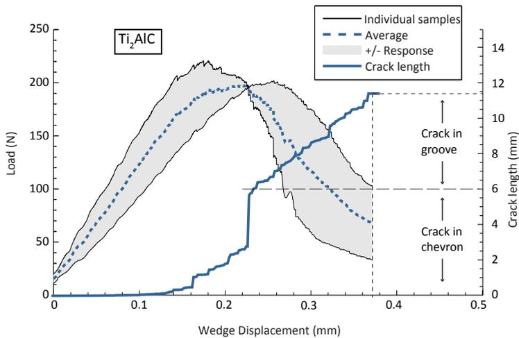
Figure 3.4: Wedge load (left axis) and normalized crack length (right axis) versus wedge displacement for  $\text{Ti}_3\text{SiC}_2$  and  $\text{Ti}_2\text{AlC}$  samples. The dashed blue line represents the average between the samples. The crack length is deduced from the acoustic energy and it is normalized using a directly measured crack length, namely (a) 9.6 mm for  $\text{Ti}_3\text{SiC}_2$  and (b) 11.36 mm for  $\text{Ti}_2\text{AlC}$ , at the end of the test.
