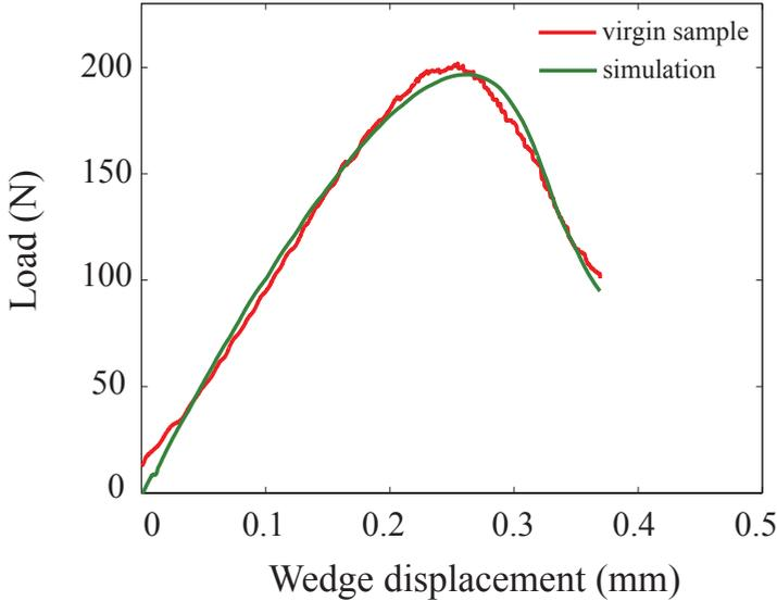
Figure 4.3: Load-displacement response of virgin specimen. Comparison between experiment and simulation. Material properties used for the simulation: fracture strength is 200 MPa, fracture energy is  $1.5 \text{ N mm}^{-1}$ , Young's modulus is 260 GPa, friction coefficient is 0.05.
