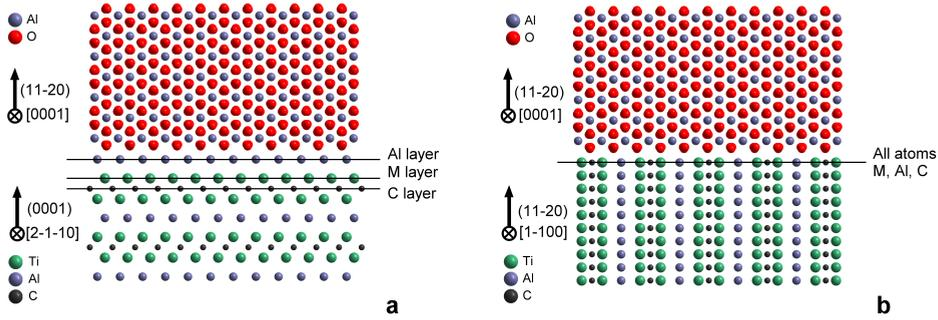
Figure 2.6: The interfaces considered are (a) MAX-phase (0001) //  $\text{Al}_2\text{O}_3$  (11-20) and (b) MAX-phase (11-20) //  $\text{Al}_2\text{O}_3$  (11-20) (b). The possible terminations of M- and A-element and C-atoms of the MAX phase are indicated by the solid lines. The composition of the (11-20) terminating plane of the MAX-phase in (b) does not change with depth and all elements are present.
