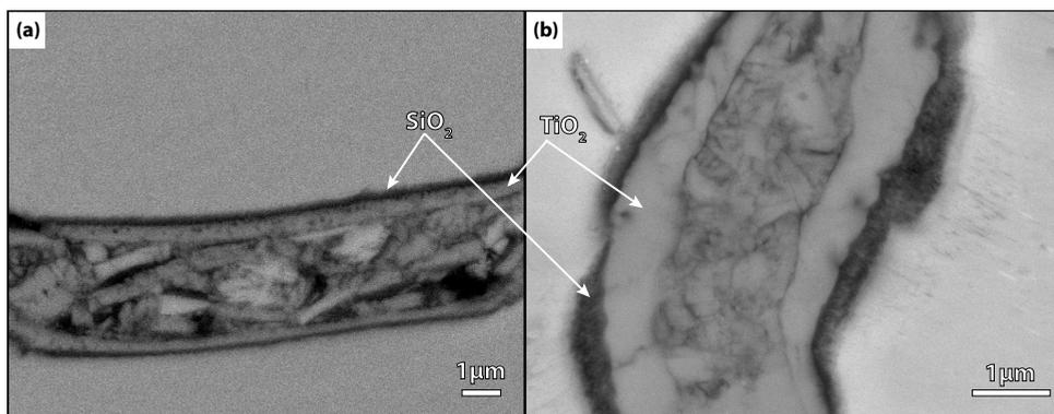
Figure 5.6: Crack in  $\text{Ti}_3\text{SiC}_2$  (a) partially filled after oxidation at  $1100\text{ }^\circ\text{C}$  for 1 h and (b) fully filled after oxidation at  $1300\text{ }^\circ\text{C}$  for 1 h.
