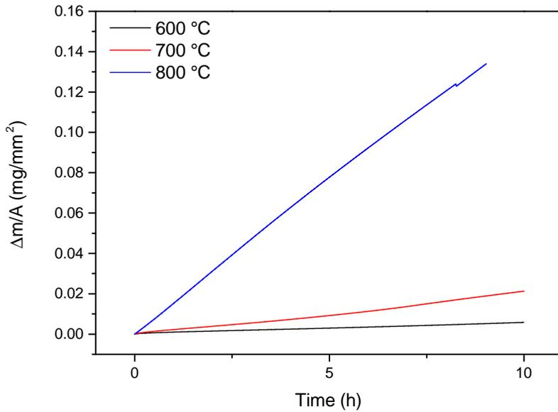
Figure 6.4: Weight gain of Ta<sub>2</sub>AlC at 600, 700 and 900°C for 10 h.
