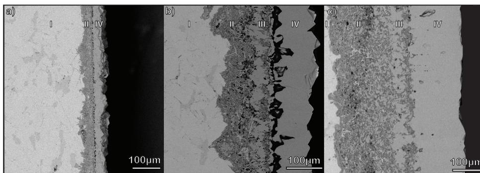
Figure 5.4: SEM backscattered electron images of cross-sectioned  $\text{Ti}_3\text{SiC}_2$ , oxidized at a) 1100 °C for 20 h, b) 1200 °C for 20 h and c) 1300 °C for 10 h; with the following phase present and marked: MAX phase (I), mixed oxides of Si and Ti (II), Ti rich oxide layer (III) and pure dense  $\text{TiO}_2$  (IV).
