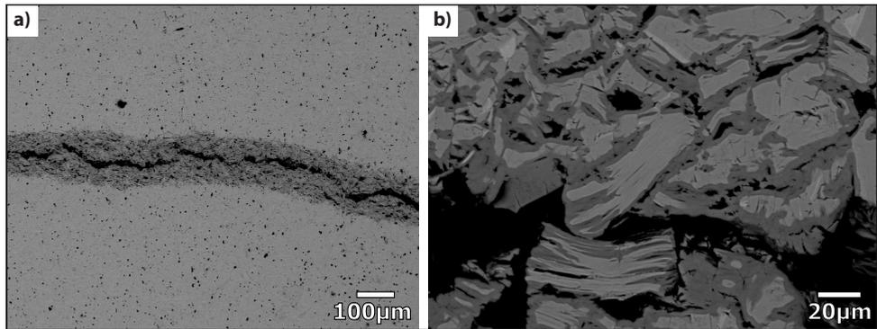
Figure 6.3: Backscattered electron image of Ta<sub>2</sub>AlC oxide after 16 h of oxidation at 600°C.
