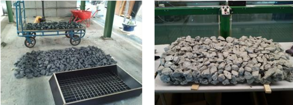
Figure 9. Toe model glued with epoxy glue (Peters, 2014)
