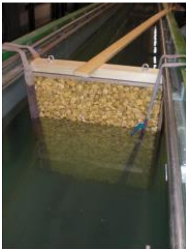
Figure 3. A piece of PBA in the flume with the location of pressure sensors (Mellink, 2012).
