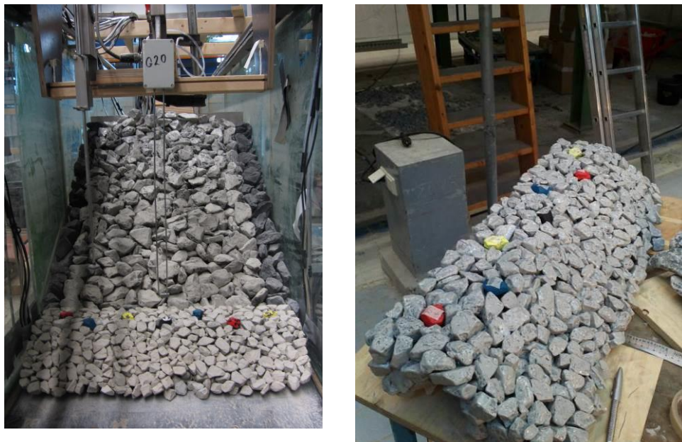
Figure 8: Glued breakwater to with six loose stones (Peters, 2014)
