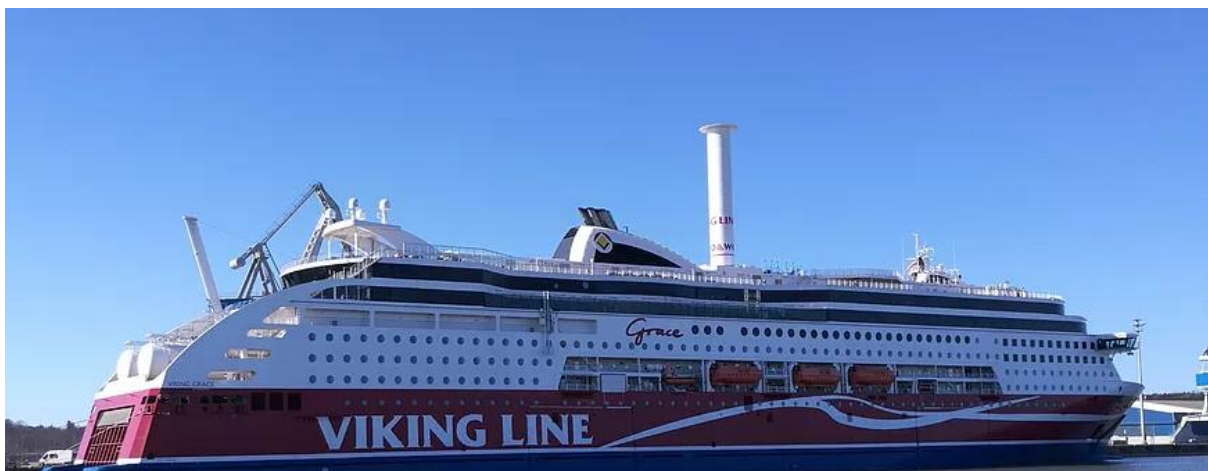
Figure 5-12: M/S Viking Grace equipped with a Flettner rotor. [205]
