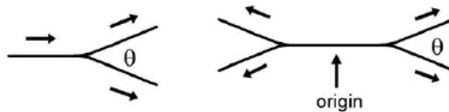
Figure 4.4: The analysis of crack branching can supply useful information [5]
