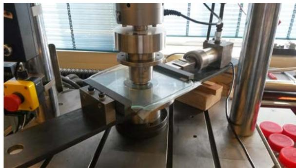
Figure 5.5: Compressive tensile test set up
