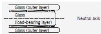
Figure 2.11: Laminated glass with sacrificial outer layers [1]
