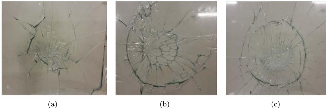
Figure 5.14: Fracture patterns of (a) CT1 (b) CT2 (c) CT3
