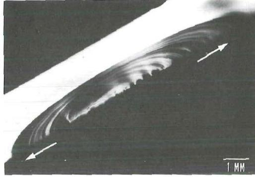
Figure 4.6: Wallner lines at the fracture origin. The arrows indicate the crack propagation direction [31]
