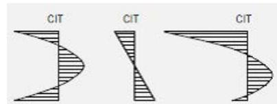
Figure 2.9: A tensile load in the outer fibers is compensated by the compressive stress [1]
