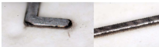
Figure 21. Electrode degradation after all experiments described in this study, performed over a span of 2 weeks (left: interfractal DBD, right: IDE DBD). Also, some discoloration of the alumina barrier can be seen, caused by prolonged CAP-induced electron etching.
