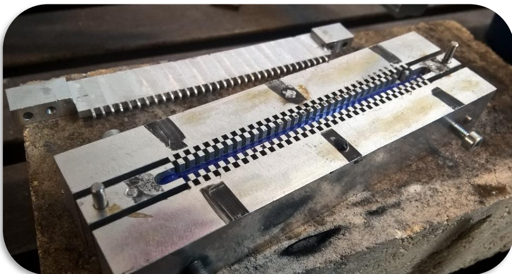
Figure 72 3-part mould used for the production of the actuator
