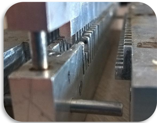
Figure 71 Top- and side-moulds partially inserted
