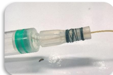
Figure 93 Reinforced seal between the silicone connector and the PEEK tubing
