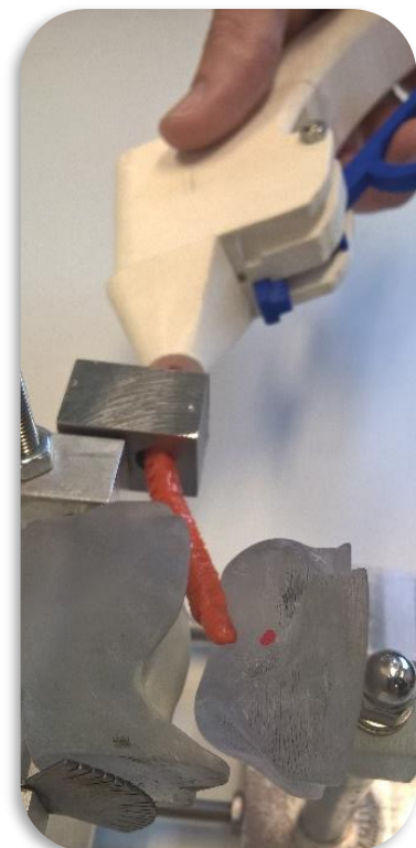
Figure 78 Artificial ankle setup with inserted actuator
