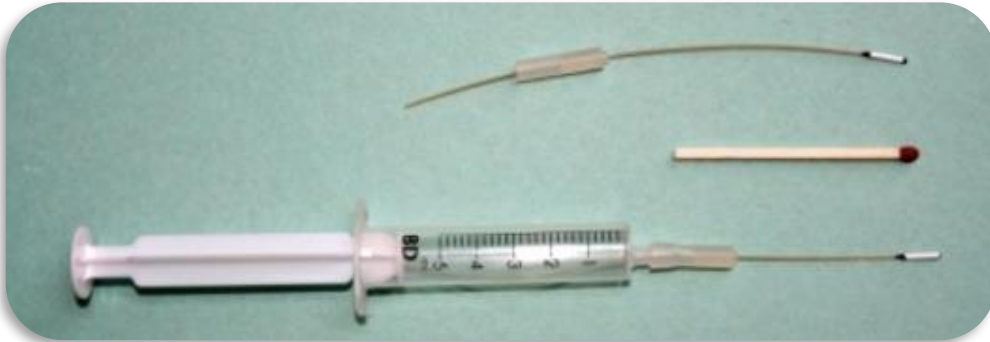
Figure 75 5ml syringe with silicone connector and PEEK tubing
