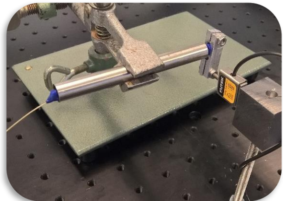
Figure 9 Rotational stiffness test setup with FPE45 actuator inserted
