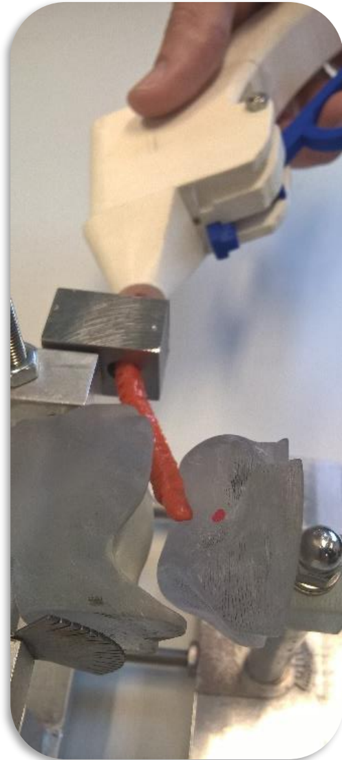
Figure 11 Artificial ankle setup with inserted actuator
