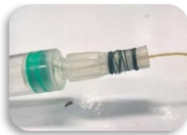
Figure 14 Reinforced seal between silicone and PEEK
