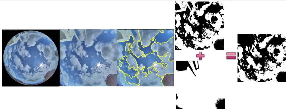
Figure 3.15: The Superpixel segmentation method explained in 5 steps. First will the ASI gets flattened. Second will the SPS method by applied. Third the mask applied. Fourth the final threshold image is made. Finally the CC % can get calculated.
