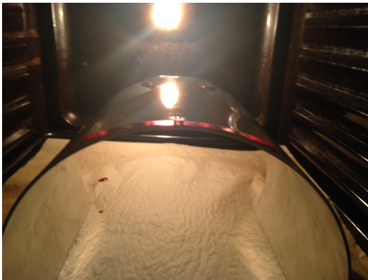
Figure B.2: At glass transition temperature the blank wraps itself around the mold radius by gravity alone, this avoids stretching of the material that happens in vacuum forming. (a), The finished shells (b) .
