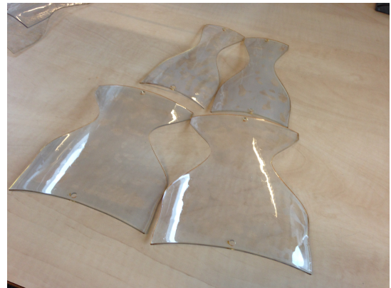
Figure B.2: At glass transition temperature the blank wraps itself around the mold radius by gravity alone, this avoids stretching of the material that happens in vacuum forming. (a), The finished shells (b) .
