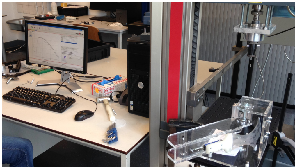
Figure C.2: The mechanism is displaced back and forth to obtain the hysteresis loop.
