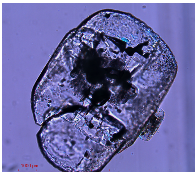
Figure 8 – Optical microscopy of a single particle showing abundant fluid inclusions
