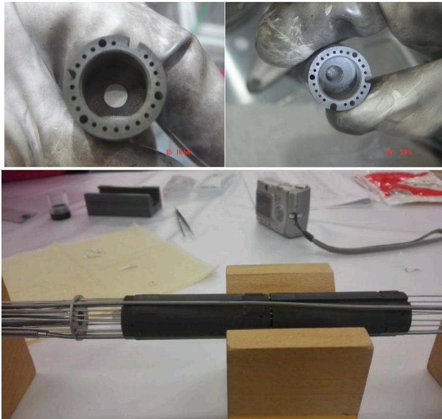
Fig. 3. Crucible loading at JRC Karlsruhe (top left: loading of the LiF-ThF 4 powder mixture, top right: same crucible after melting), and assembly of sample holder at NRG (bottom).
