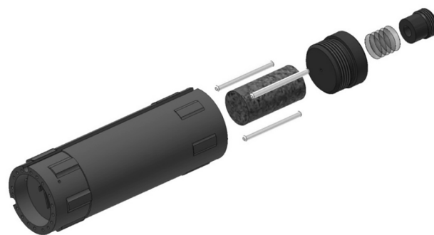
Fig. 2. Exploded view of crucible (diameter \sim 22\text{ mm} , length 80\text{ mm} ), showing from left to right: the crucible, the salt column, 3 activation monitor sets, the end cap, a metallic filter prepared from a stack of stainless steel wire meshes, and the filter cap. The crucible walls contain additional holes for thermocouples and gas lines.
