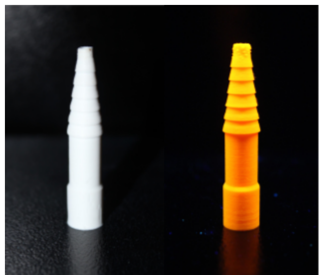
Figure 3: Left: White ABS connector; Right: Orange PETG connector;
