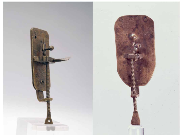
Fig. 1. The two original Van Leeuwenhoek microscopes that were studied with neutron tomography. The lens sits mounted between the brass plates, at the position of the specimen pin. (A) A medium-powered ( \times 118 ) instrument (Rijksmuseum Boerhaave, Leiden, inventory number V7017). Note that there is a redundant drill hole in the upper left corner of the instrument, not to be confused with its lens aperture, which is directly behind the pin. This microscope is numbered #1 by Van Zuylen. Photo credit: Tom Haartsen Fotografie, Ouderkerk aan de Amstel. (B) The instrument with the highest magnification among the preserved ones ( \times 266 ) (Utrecht University Museum, inventory number UM-1). This microscope is numbered #3 by Van Zuylen. Photo credit: Utrecht University Museum.
