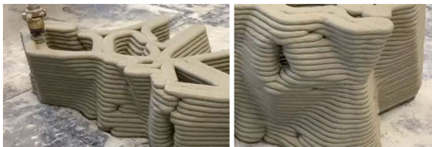
Fig. 3.1 Rhizome 1.0 prototypes using Vertico's cement-based concrete and robotic system
