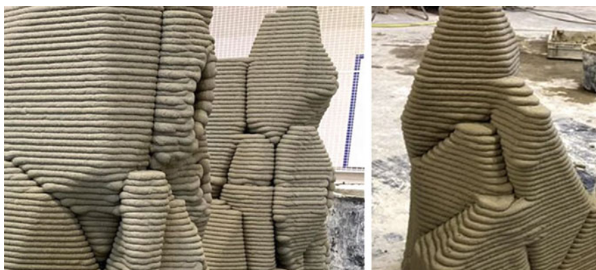
Fig. 3.6 Stackable 3D printed components
