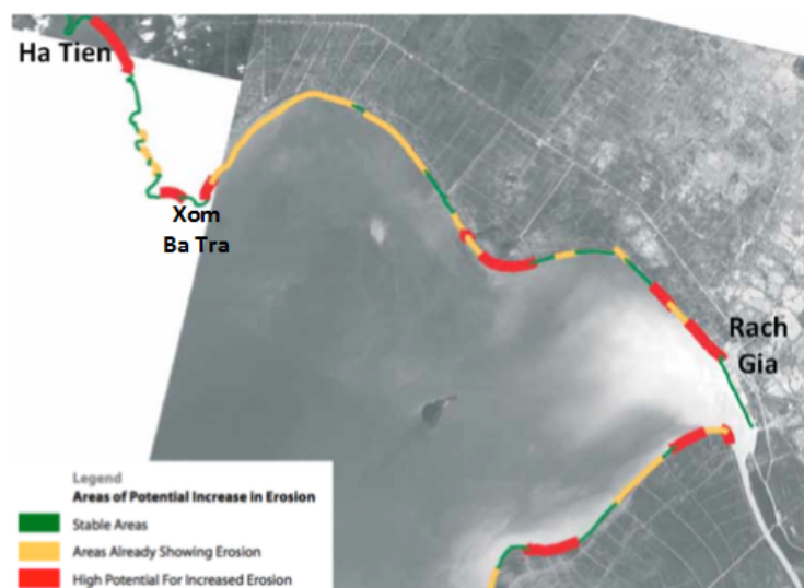
Figure 4-6 Coastal erosion indication between the Ha Tien and Rach Gia. Red = High potential increase erosion, Yellow = signs of erosion and green = stable areas.
