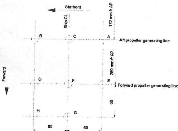
Figure 11: Pressure transducers arrangement
