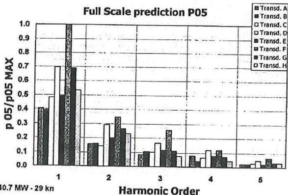
Figure 12: Measured pressure pulses
