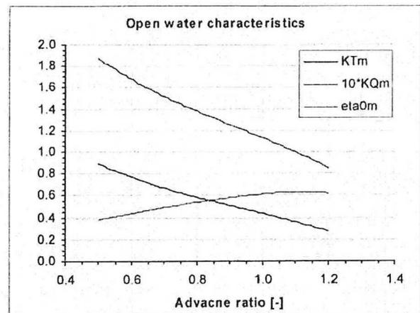
Figure 4: Propeller characteristics
