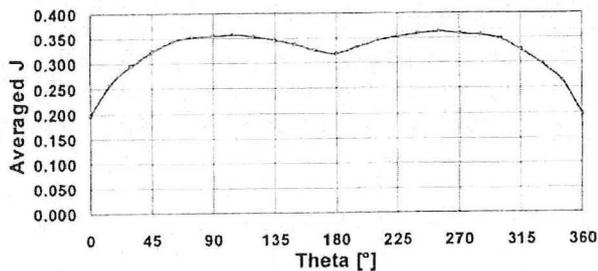
Figure 14: Forward propeller advance coefficient distribution on the wake field measurements
