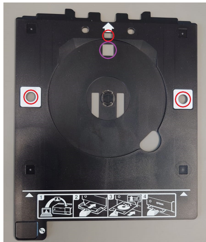
Figure 3.2: Stock CD tray. Holes marked in red have to be unobstructed and the hole marked in purple has to be obstructed in order for the printer to accept the tray.
