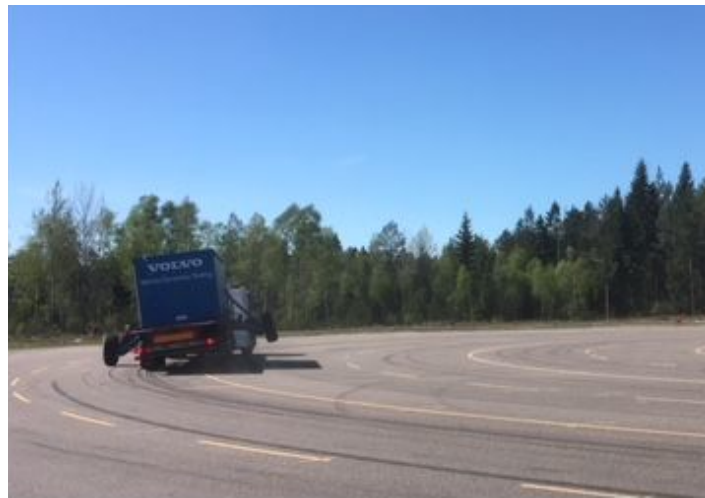
Figure 7-2: Photo of the truck during performing a rollover on the skidpad
