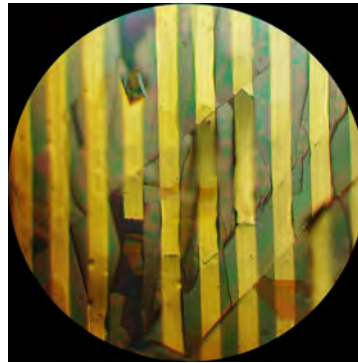
(b) The cracks combined with damage to the surface cause the electrodes to lift off the chip
